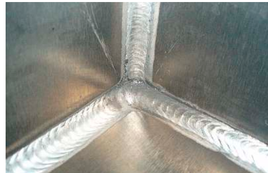
Fig. 12 Bead appearance welded by robot
