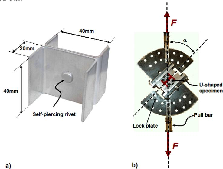
Fig. 5: a) Geometry of U-shaped specimens, and b) Testing facility
