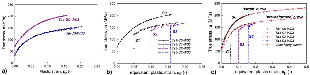
Fig. 4: Material properties, a) Stress-strain curves of alloy 6063W at different aging times, b) Tension-tension results from tensile testing of pre-stretched material in temper W-10min (denoted by W00) and subjected to natural aging for 3days (denoted by W03), c) Representative stress-strain curves of 'virgin' and 'pre-deformed' materials
