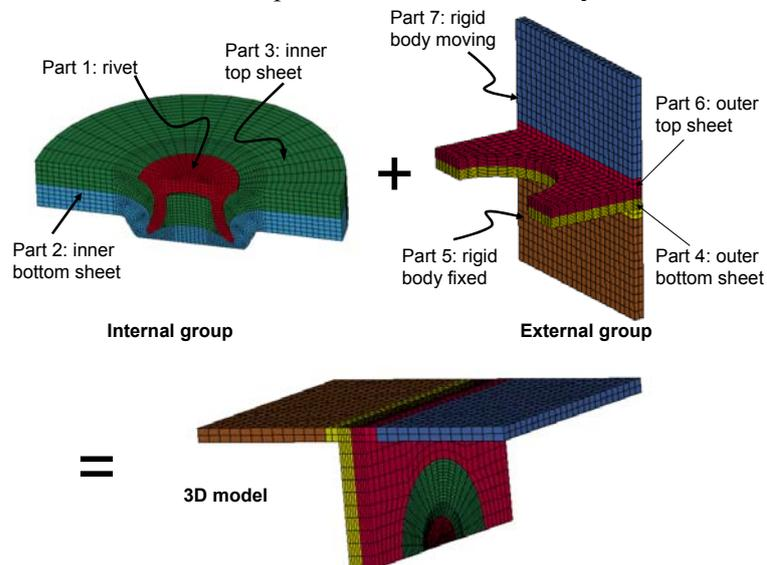
Fig. 6: A half of 3D model of the riveted connection
