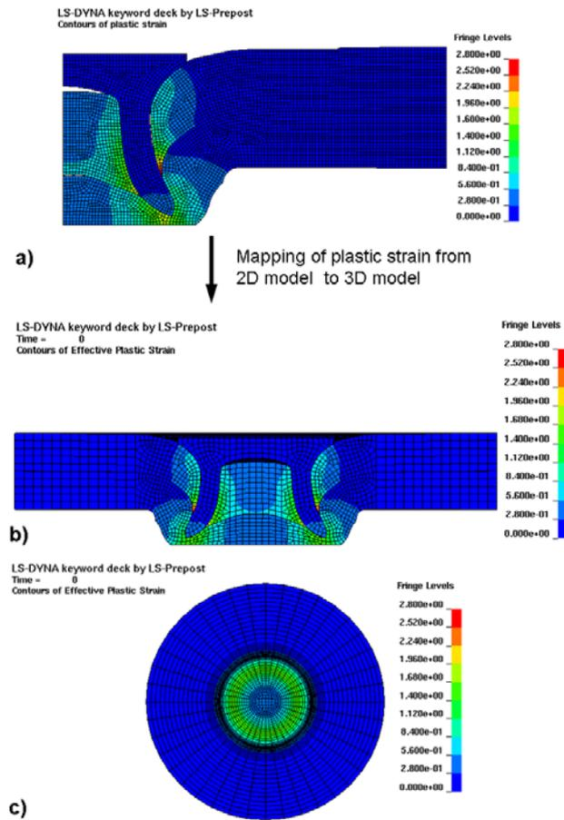
Fig. 7: Mapping process: a) results from the 2D riveting process analysis with fine mesh, b) 3D model generated with a coarser mesh including the stress-strain distribution from the 2D analysis, and c) a view from bottom of the 3D model – all the elements situated on the same circumference and z-coordinate have the same value of the initial stress and strain
