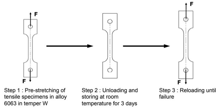
Fig. 3: Material testing procedure
