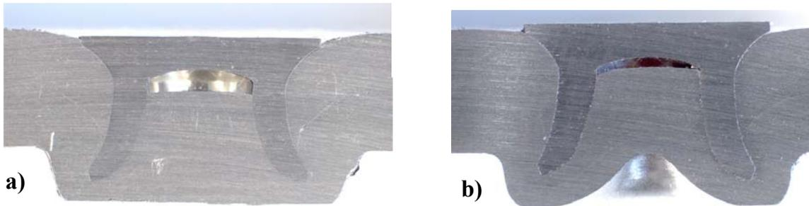
Fig. 2: Cross-sections of proper riveted connections by using aluminium rivets in alloy 7278-T6, a) FM die, b) DZ die.
