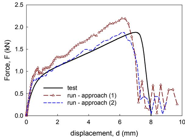
Fig. 9: Comparison between experimental and numerical force-displacement curves of aluminium riveted connections under pure pull-out loading condition with different modelling strategies
