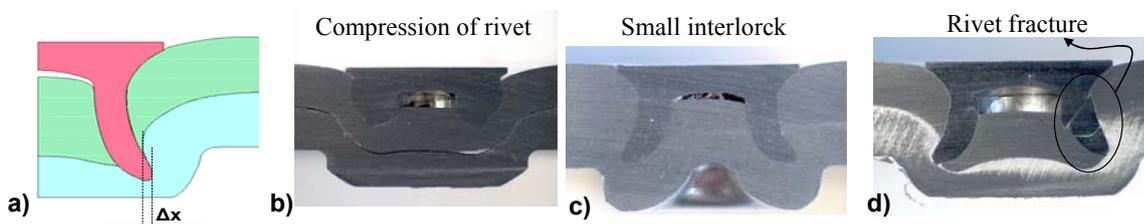
Fig. 1: Joining of aluminium plates by using an aluminium rivet, a) definition of the mechanical interlock, b) compression of the rivet, c) small interlock, d) fracture in rivet
