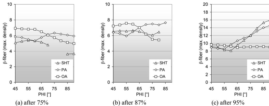
Fig. 2 Cold rolling textures after 75, 87 and 95% thickness reduction for three different solution / precipitation conditions (see Fig. 1); the cold rolling textures are represented by means of the skeleton line along the  $\beta$ -fiber
