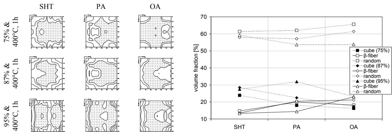
Fig. 3 Recrystallization textures for three different solution / precipitation states achieved after annealing at 400°C for 1h (see Fig. 1); the textures are represented by  $\phi_2 = 0^\circ$  sections (Levels: 1.2 / 2 / 4 / 7 / 12) and in terms of volume fractions for respective texture components
