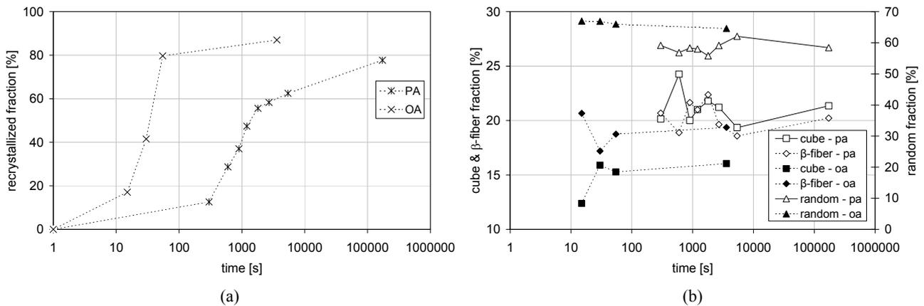
Fig. 4 (a) Recrystallization kinetics from EBSD data for the PA and OA sample which were cold rolled to 75% thickness reduction and annealed at 300°C; (b) texture evolution of recrystallized grains for both material conditions, the textures are represented in terms of volume fractions for respective texture component groups
