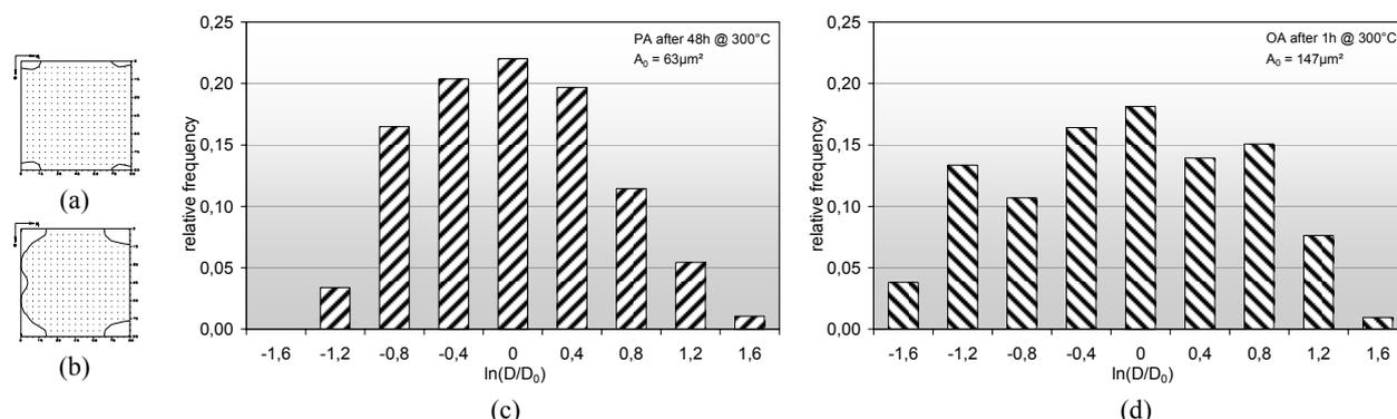
Fig. 6 (a) Experimental recrystallization texture for OA material after 75% cold rolling and annealing at 400°C for 1h, (b) corresponding simulated recrystallization texture; the textures are represented by  $\phi_2 = 0^\circ$  sections (Levels: 2 / 4); experimental size distribution of recrystallized grains: (c) for PA after 48h at 300°C and (d) for OA after 1h at 300°C
