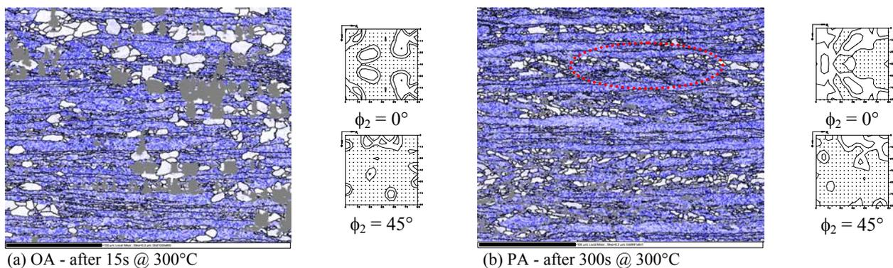
Fig. 5 Partially recrystallized microstructures and corresponding ODFs of recrystallized grains only: (a) over-aged condition, (b) peak-aged condition
