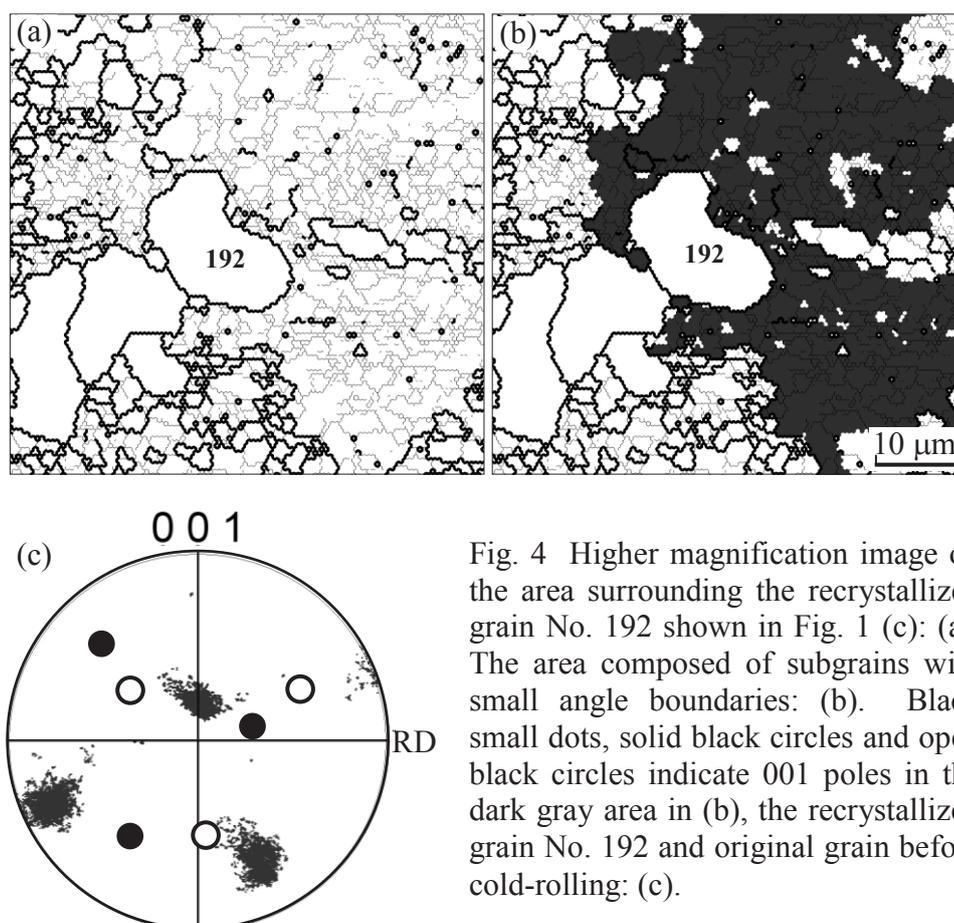
Fig. 4 Higher magnification image on the area surrounding the recrystallized grain No. 192 shown in Fig. 1 (c): (a). The area composed of subgrains with small angle boundaries: (b). Black small dots, solid black circles and open black circles indicate 001 poles in the dark gray area in (b), the recrystallized grain No. 192 and original grain before cold-rolling: (c).
