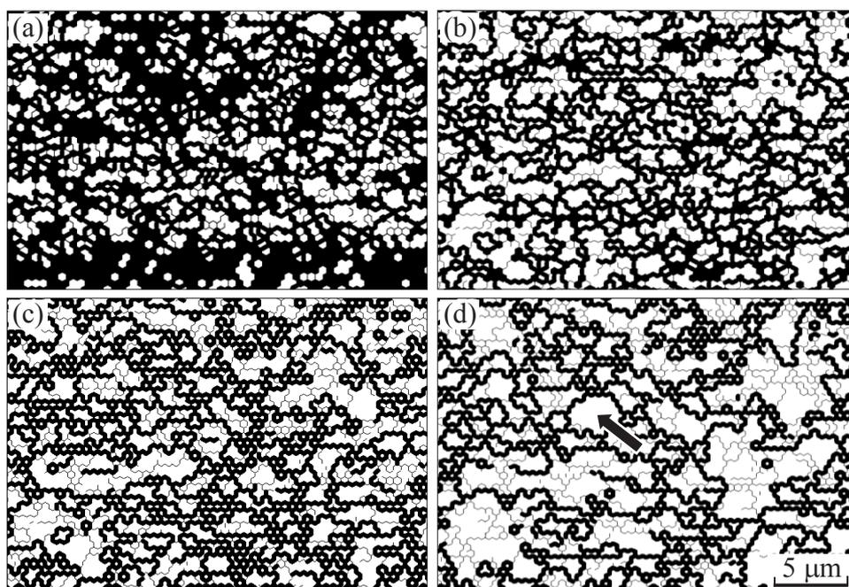
Fig. 2 Microstructures in after cold-rolled at 50 % (a), and changes in microstructures in the early stage of annealing at 673 K for 6 s, 10 s, and 20 s, (b), (c) and (d), respectively. The black arrow in (d) indicates the crystallite for the recrystallized grain No. 192.
