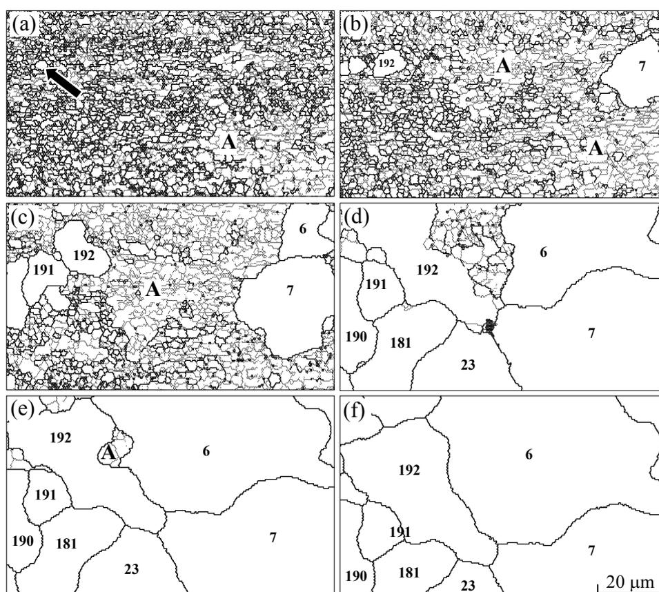
Fig. 1 Changes in microstructures during annealing at 673 K for 20 s, 40 s, 60 s, 120 s, 0.6 ks and 1.8 ks, (a) to (f), respectively after cold-rolled at 50 %. The black arrow in (a) indicates the crystallite for the recrystallized grain No. 192.
