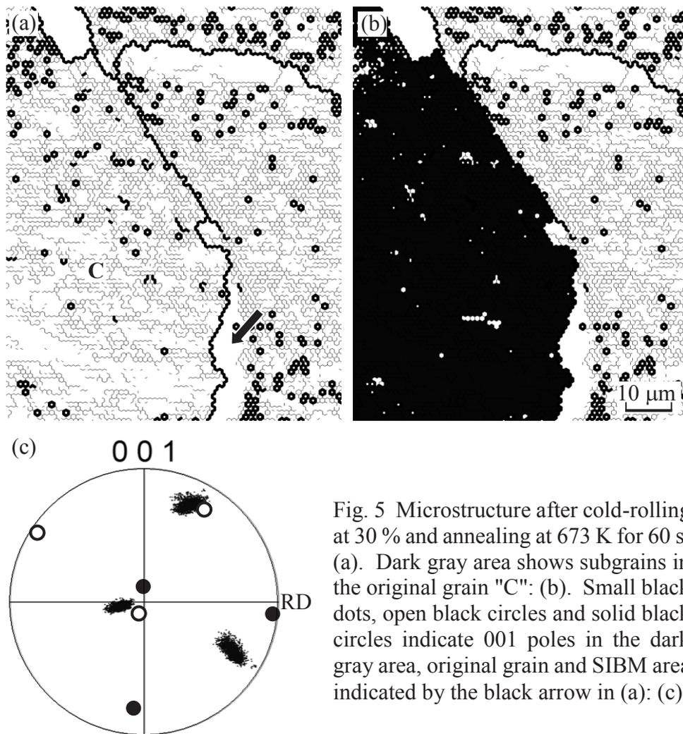
Fig. 5 Microstructure after cold-rolling at 30 % and annealing at 673 K for 60 s: (a). Dark gray area shows subgrains in the original grain "C": (b). Small black dots, open black circles and solid black circles indicate 001 poles in the dark gray area, original grain and SIBM area indicated by the black arrow in (a): (c).
