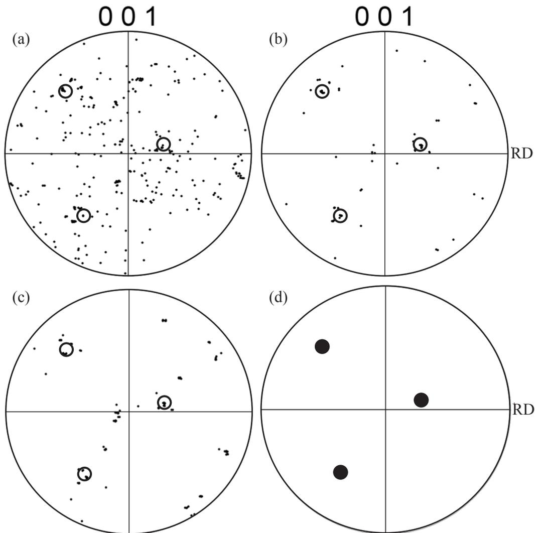
Fig. 3 (001) poles in the area around the crystallite for the recrystallized grain No. 192 indicated in Fig. 2 (d) in the as-rolled condition, annealed at 673 K for 6 s, 10 s and 20 s, (a) to (d), respectively. Black solid circles in (d) and open circles in (a), (b) and (c) indicate the (001) pole of the No. 192 grain.
