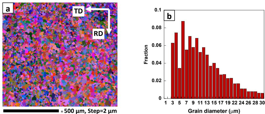
Fig. 2. (a) EBSD map showing recrystallized grain structure of *NA-CR-380* in the rolling plane, (b) Average grain diameter distribution for the EBSD map.
