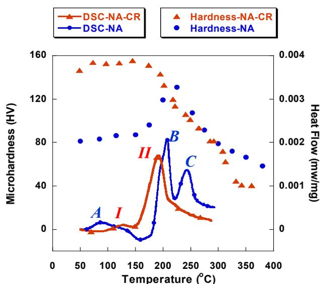
Fig. 5. DSC thermograms and hardness evolution of naturally aged and cold rolled (*NA-CR*), and naturally aged (*NA*) samples.
