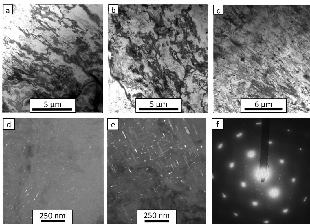
Fig. 3. Bright field (a-c) and dark field (d, e) TEM micrographs in  $[001]_{Al}$  projection of (a) *NA-CR*, (b, d) *NA-CR-180* and (c, e) *NA-CR-235* samples; (f) A SADP obtained from *NA-CR-235* at  $[001]_{Al}$  zone axis.
