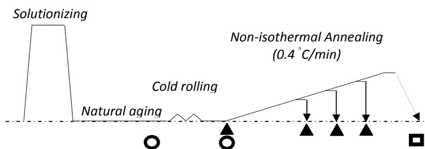
Fig. 1. Schematic presentation of the processing routes used for preparing the DSC (○), TEM (▲) and EBSD (■) samples.
