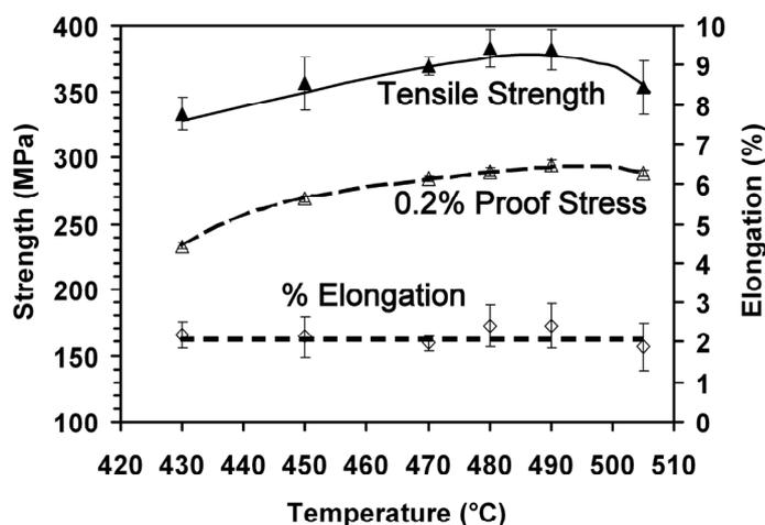
Fig. 2. Tensile properties of the ADC12 alloy studied as a function of solution treatment temperature.
