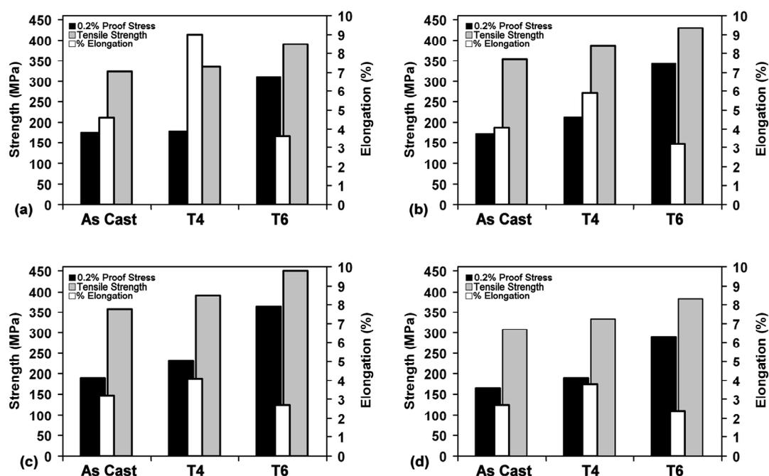
Fig. 1. Tensile properties of the four alloys made from cylindrical tensile test bars examined in as-cast, T4 and T6 tempers. (a), ADC3, (b), ADC10#1, (c) ADC10#2, (d) ADC12.
