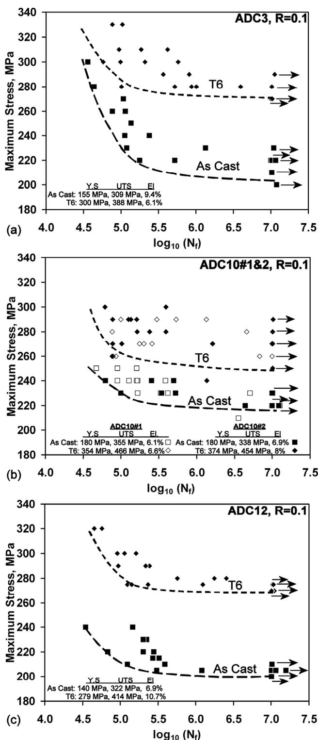
Fig. 4. Axial  $S-N_f$  data,  $R = 0.1$ . in as-cast and T6 conditions (a) shows ADC3, (b) shows ADC10 and (c) shows ADC12. Data at  $10^7$  cycles are runouts.
