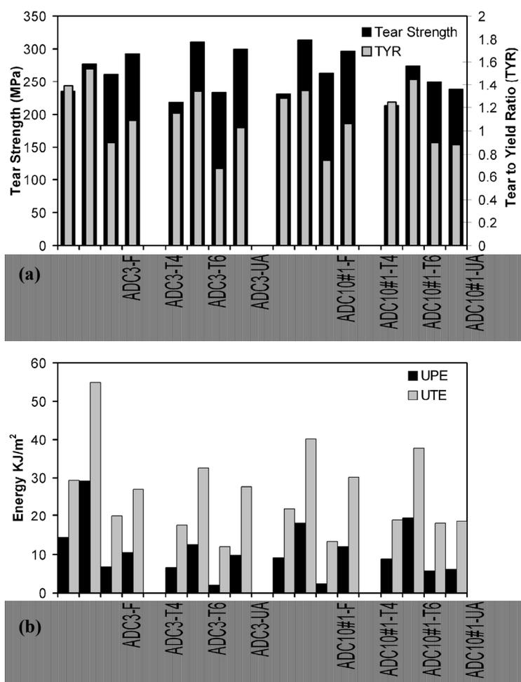
Fig. 3. a) shows tear strength and tear-to-yield ratio for the four alloys; b) shows the unit propagation energy, (UPE) and unit total energy (UTE).
