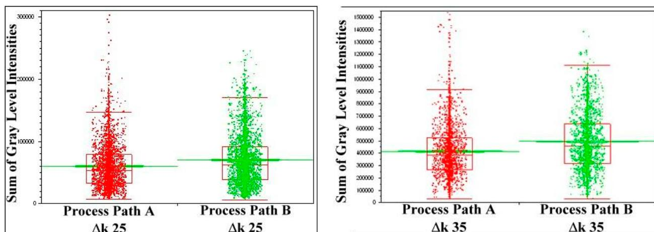
Fig. 6 Weighted particle area within plastic zones for two different processing path at two different  $\Delta k$ s a)  $\Delta k=25$  MPa $\sqrt{m}$  b) for  $\Delta k=35$  MPa $\sqrt{m}$
