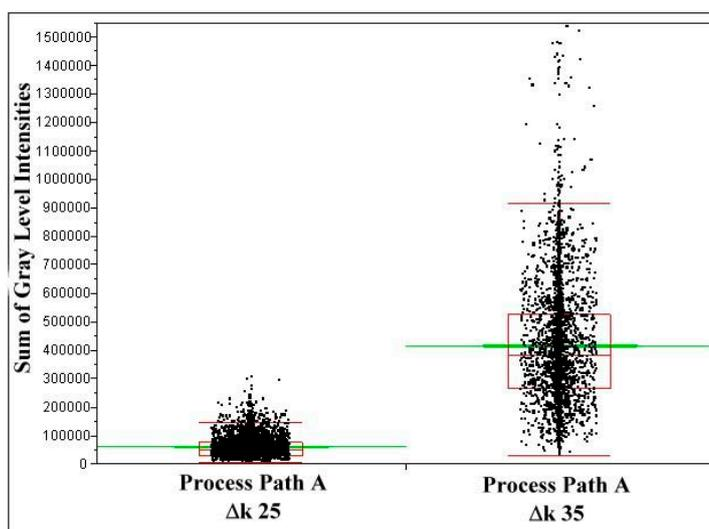
Fig. 5 Scatter plot of summed intensities for two different plastic zone sizes, based on the analysis of the microstructure created in processing path A
