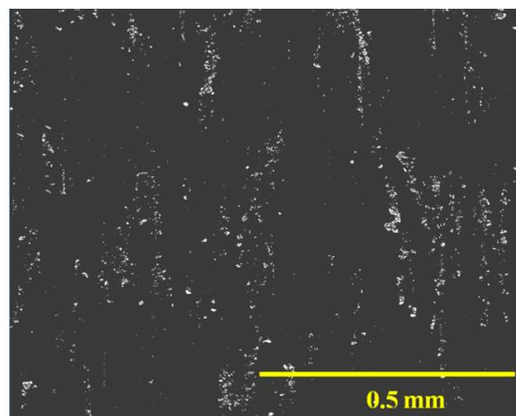
Fig 3: Constituent particles characterized by BSE-SEM in the rolling plane at mid-thickness of the sheet. A subset of 5x3 frames of the whole area analyzed is shown.
