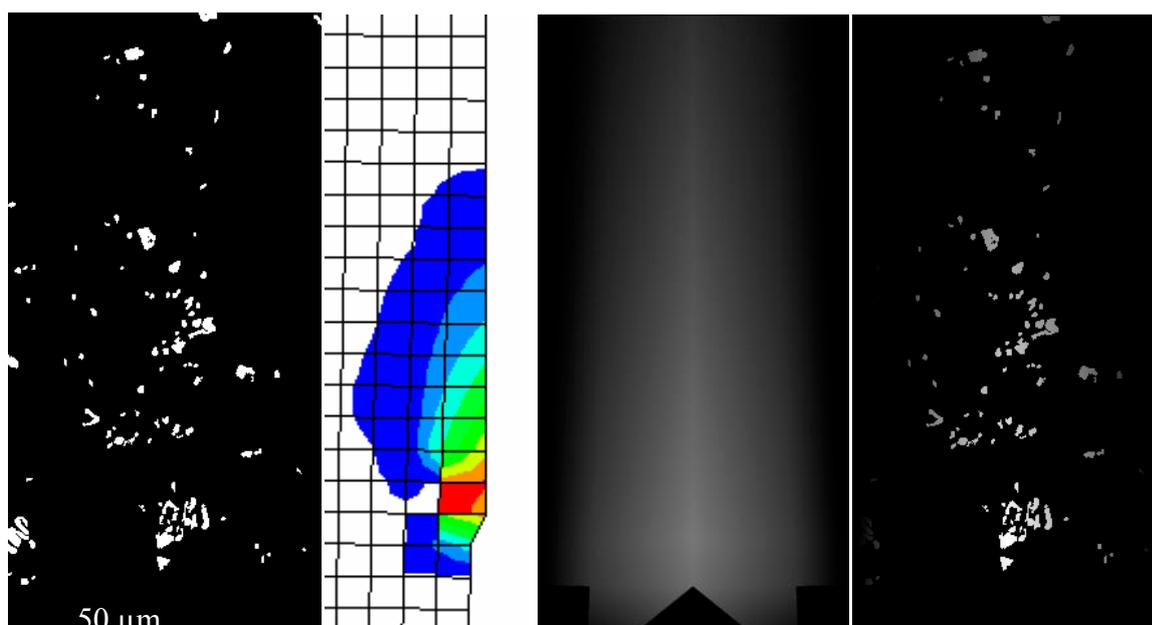
Fig 4: Applying FEM-based plastic zone shape to the images of second phase particles
