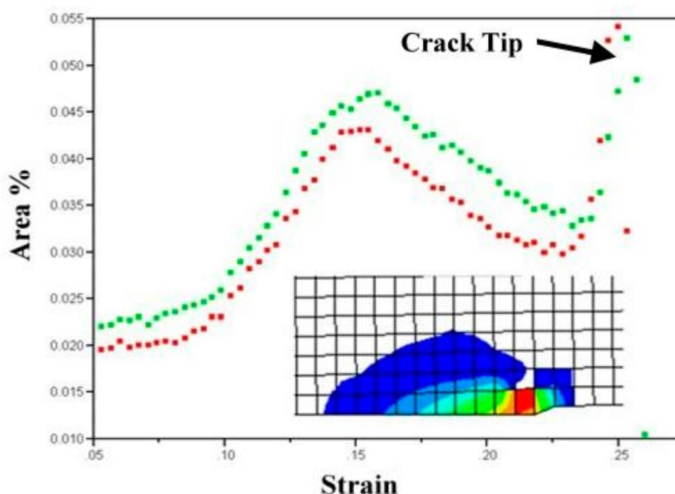
Fig. 7 Area fraction of constituent particles at different strain levels within the simulated plastic zone for a  $\Delta k$  of 25 MPa $\sqrt{m}$ . Upper curve (green) are data for processing path A, lower curve (red) are data for processing path B. For illustration purpose, Fig 4 b is pasted into the graph in the orientation of the data on the X-axis.
