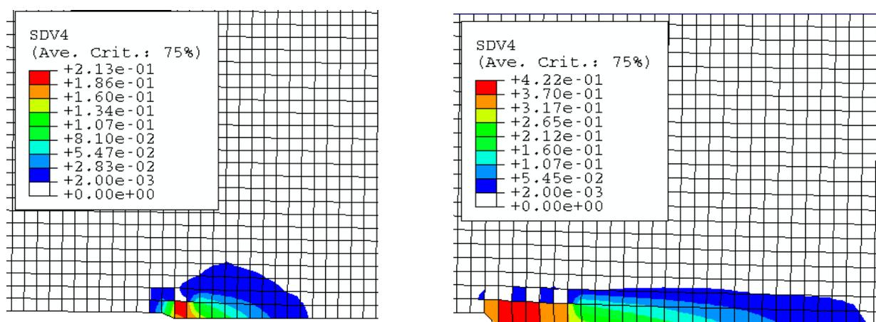
Fig 2: Incremental change in plastic zone size between two load cycles during fatigue testing from FE simulation at two different  $\Delta k$ : a)  $25 \text{MPa}\sqrt{\text{m}}$  b)  $35 \text{MPa}\sqrt{\text{m}}$
