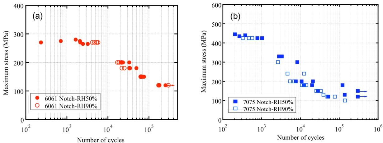
Fig.1 S-N curves of 6061 and 7075 alloys (Notch, frequency: 1.0 Hz, stress ratio: 0.1)
