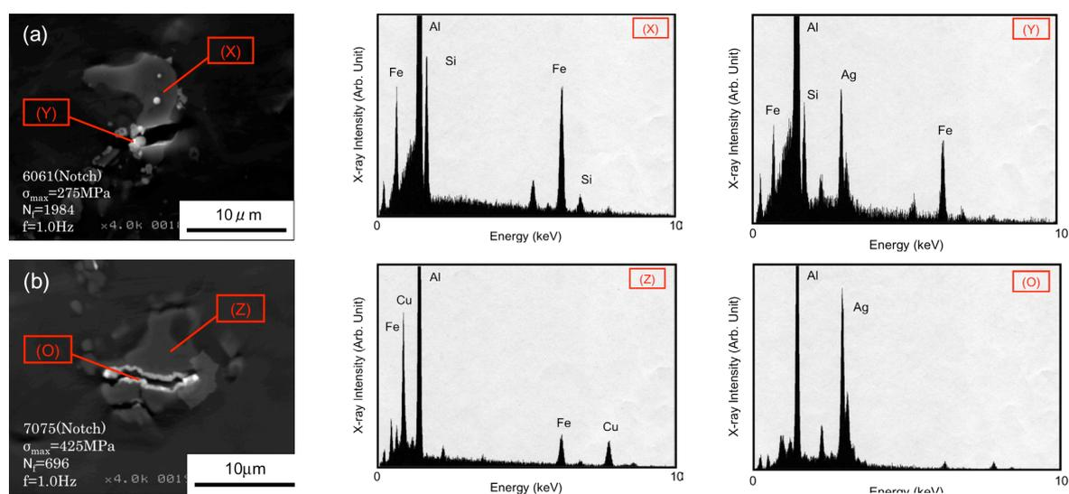
Fig.6 HMT/EDX images after the fatigue fracture in the specimens, (a) 6061(Notch), (b) 7075(Notch), in which the frequency was 1.0 Hz.
