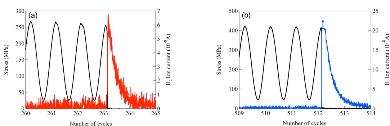
Fig.4 Hydrogen evolution behavior in the fatigue fracture with a test frequency of 1.0 Hz, (a) 6061(Notch), (b) 7075(Notch).
