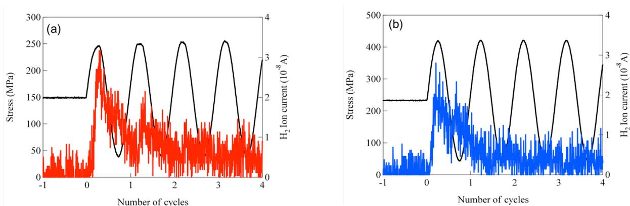
Fig.3 Hydrogen evolution behavior in the fatigue with a test frequency of 1.0 Hz, (a) 6061(Notch), (b) 7075(Notch).
