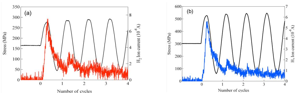
Fig.2 Hydrogen evolution behavior in the fatigue with a test frequency of 1.0Hz, (a) 6061(Smooth), (b) 7075(Smooth).
