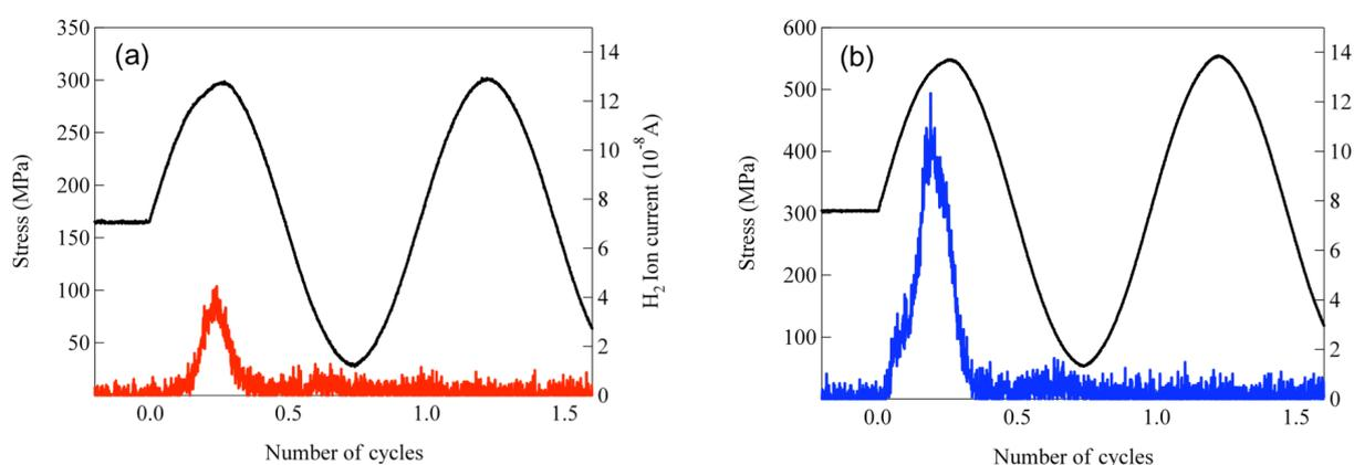
Fig.5 Hydrogen evolution behavior in the fatigue with a test frequency of 0.1 Hz, (a) 6061(Smooth), (b) 7075(Smooth).
