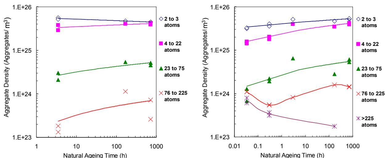
Fig. 5: Effect of natural ageing on the density of differently sized solute aggregates in (a) T4 and (b) T6 conditions, based on the number of aggregates per box divided by the box volume ( $N = 2$ ).
