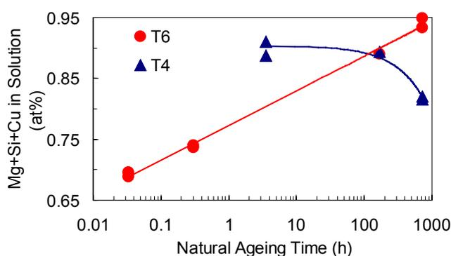
Fig. 6: Effect of natural ageing on amount of solute in solution as determined by using  $N = 2$ .
