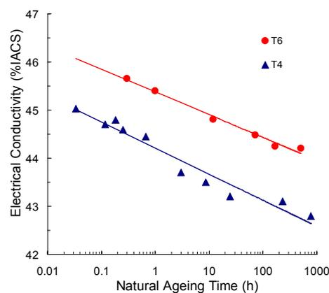
Fig. 2: Effect of natural ageing on the electrical conductivity.
