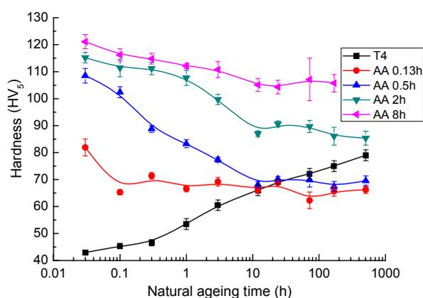
Fig. 1: Effect of natural ageing time on the hardness before and after ageing at 170 °C.
