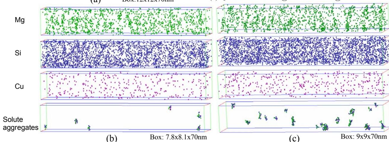
Fig. 4: 3DAP elemental maps in different conditions, showing Mg, Si and Cu atom distributions, and corresponding maps of solute aggregates resolved using particle analysis parameters of  $D = 0.5$  nm,  $L = 0.5$  nm,  $S = 0.5$  nm and  $N = 10$  atoms. Heat treatments for (a) (b) and (c) are specified in Table 2.
