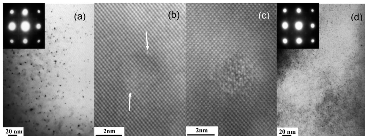
Fig. 3: Bright-field TEM and HRTEM micrographs along the  $[001]_{Al}$  direction in different ageing conditions: (a) Quenched + 0.03 h@20 °C + 0.5 h@170 °C, (b) HRTEM of (a) showing a coherent zone, (c) HRTEM of (a) showing a  $\beta''$  precipitate, (d) Quenched + 168 h@20 °C + 0.5 h@170 °C.
