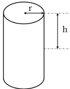
**Fig. 1:** Schematic representation of the assumed cylindrical morphology for precipitates
