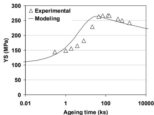
**Fig. 3:** Prediction of the yield strength of the alloy AA6061 aged at 170 °C.
