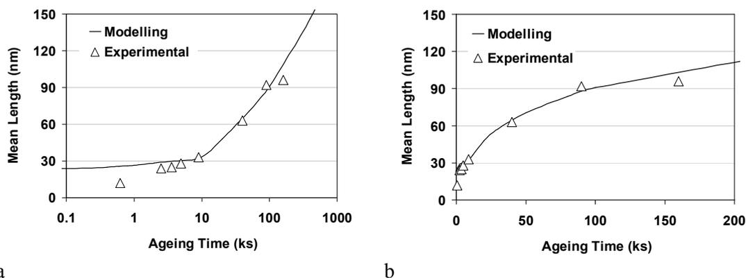
**Fig. 2:** Prediction of the length of precipitate in the alloy AA6061 aged at 190 °C in the a) Log-scale and b) linear scale
