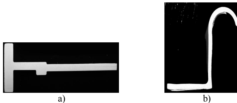
Fig.2 Cross-section of 1445 alloy sections: a) wall thickness is 8 mm; b) wall thickness is 1.5 mm;
