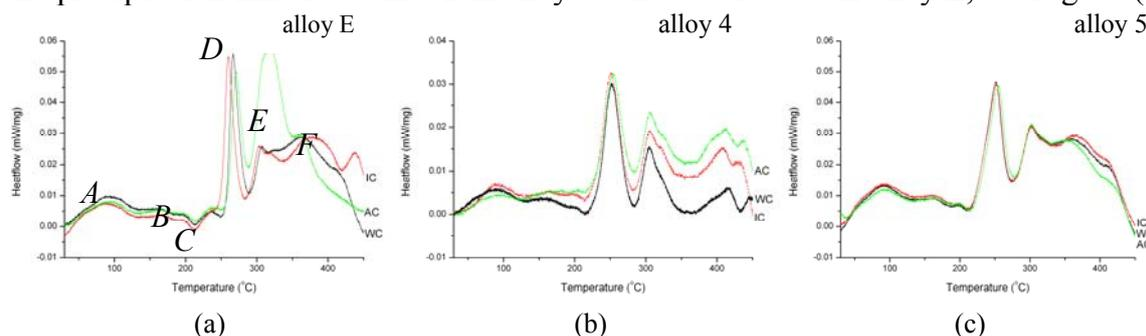
Fig. 4. DSC traces measured at 10 K/min heating rate after quenching in different media of (a) alloy E, (b) alloy 4, (c) alloy 5.
