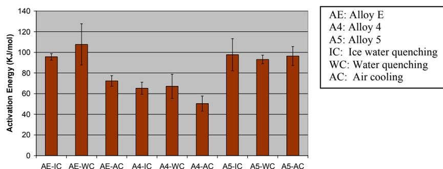
Fig. 5. Activation energy of  $\beta''$  formation (IC= ice-water cooling, WC= ‘room temperature’ water cooling, AC=air cooling).
