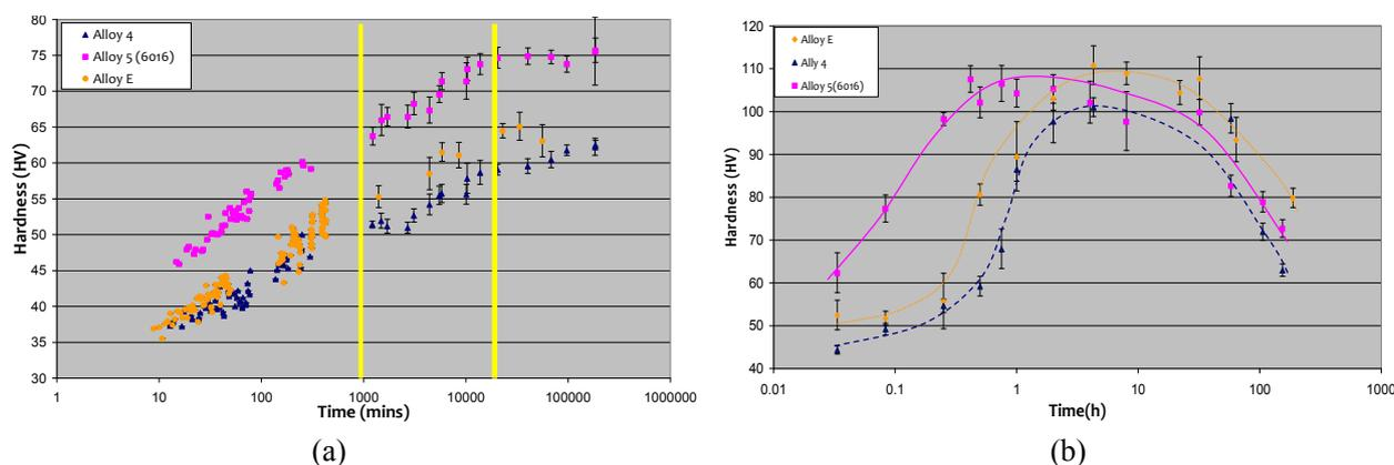
Fig. 1. Hardness evolution during (a) natural ageing (b) immediate artificial ageing of the three alloys after solutionising and quenching in ice water.
