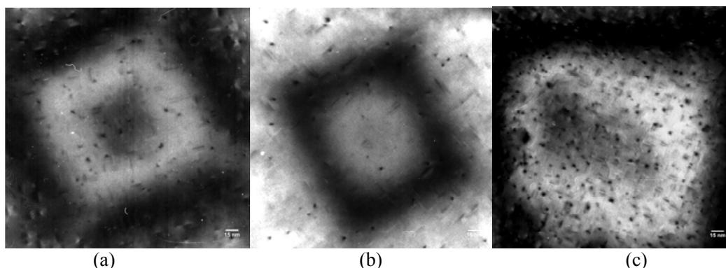
Fig. 3. TEM bright field images and of samples in the paint baked condition (1hr SHT@540 + 20min AA@180 °C).
