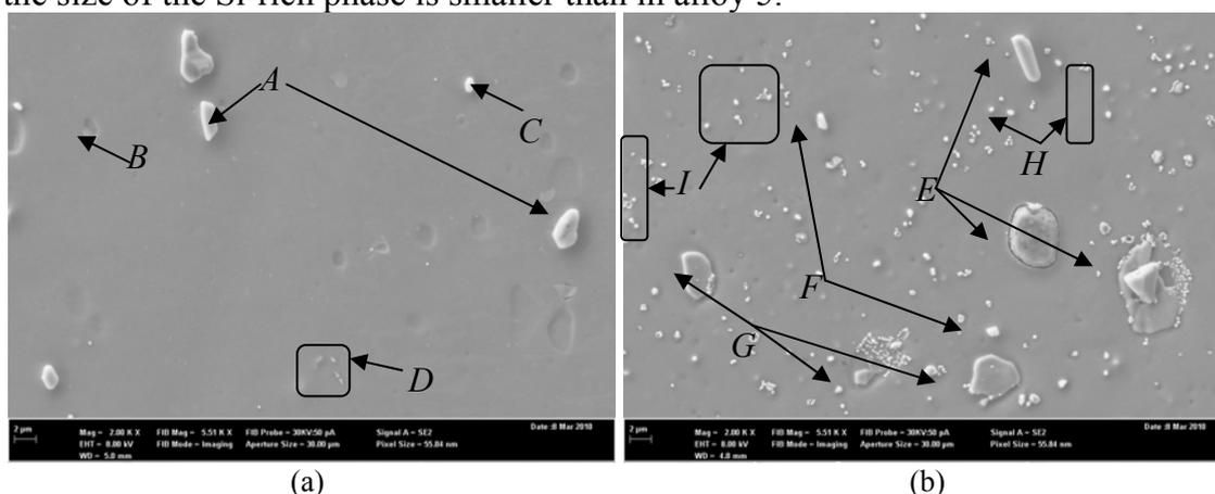
Fig. 2. SEM images of (a) alloy 4 and (b) alloy 5 showing intermetallic phases
