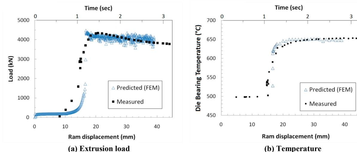
Fig. 3 - Validation of simulation results for: a) Extrusion load and b) Temperature (Homogenization treatment prior to extrusion:  $550^\circ\text{C}$  for 8h, Extrusion temperature =  $550^\circ\text{C}$ ).
