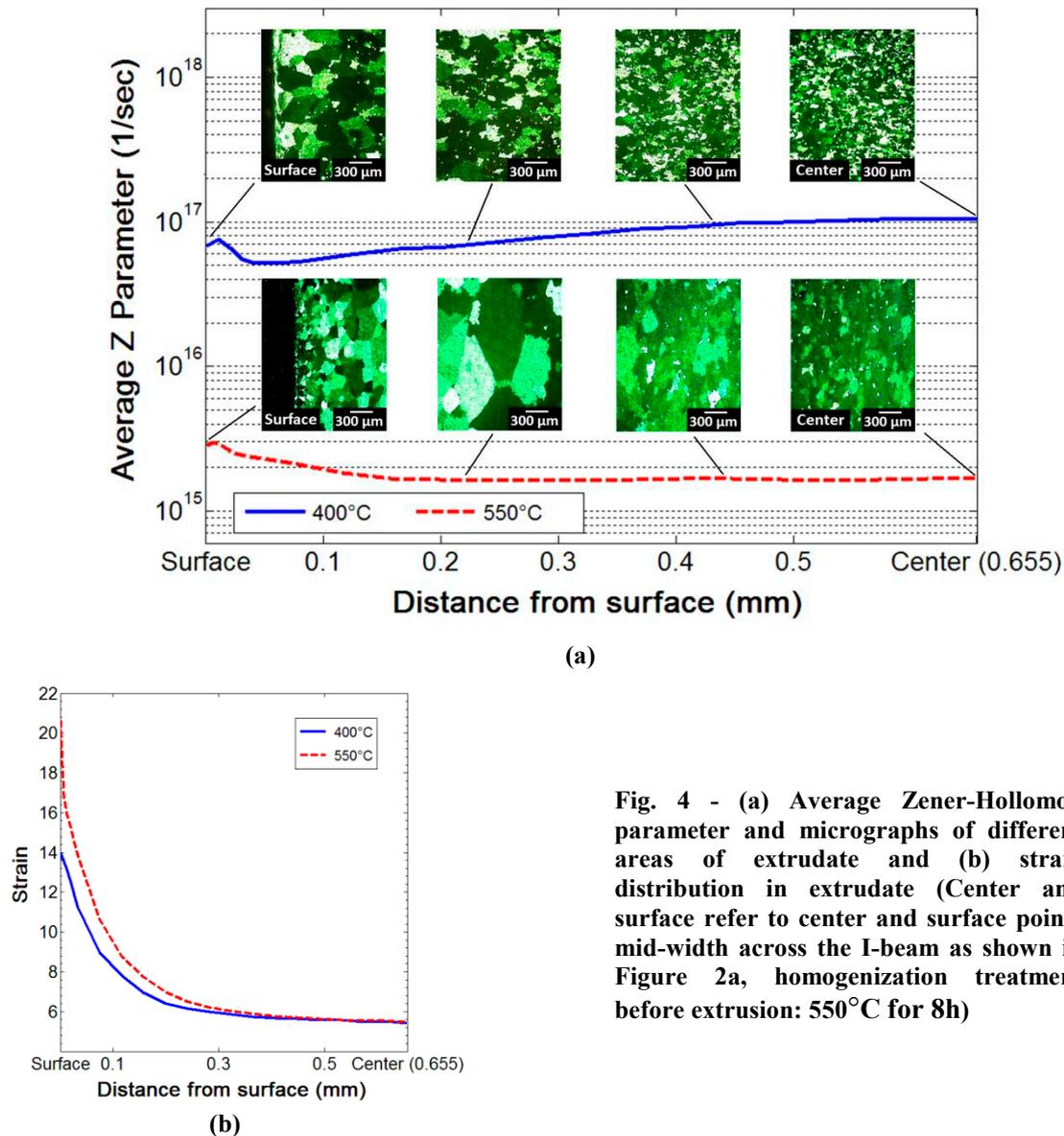
Fig. 4 - (a) Average Zener-Hollomon parameter and micrographs of different areas of extrudate and (b) strain distribution in extrudate (Center and surface refer to center and surface points mid-width across the I-beam as shown in Figure 2a, homogenization treatment before extrusion:  $550^\circ\text{C}$  for 8h)
