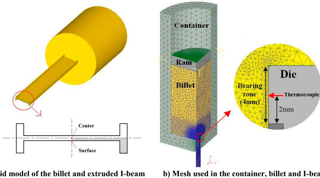
a) Solid model of the billet and extruded I-beam      b) Mesh used in the container, billet and I-beam
