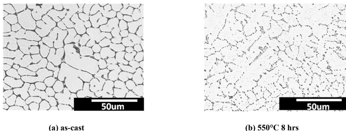
**Fig. 1 - Homogenized microstructure for billets given: a) as-cast and b) 550°C for 8 hrs**
