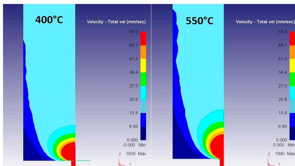
Fig. 5 - Calculated flow velocity for material extruded at 400°C (left) and 550°C (right).
