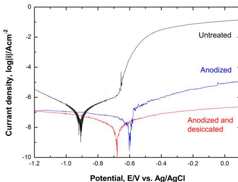
Fig. 7 Potentiodynamic polarization curves of three different treated samples in  $0.6 \text{ kmolm}^{-3}$  NaCl.
