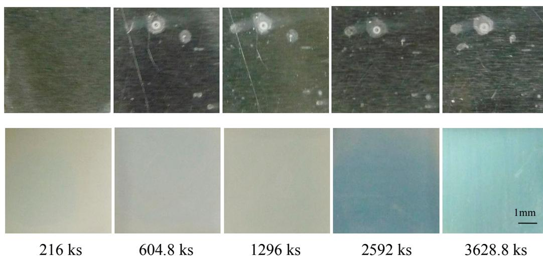
Fig. 5 The surface appearance of untreated sample (above) and hydrophobic sample (below) changes with immersion time in  $0.6 \text{ kmolm}^{-3} \text{ NaCl}$ .
