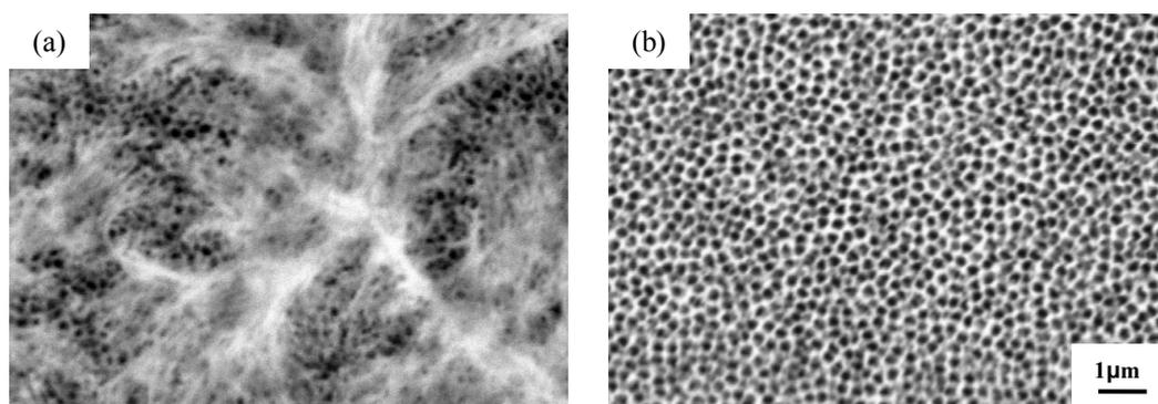
Fig. 2 SEM photos of sample surface after anodizing (a) and after desiccation at 393 K for 43.2 ks (b).
