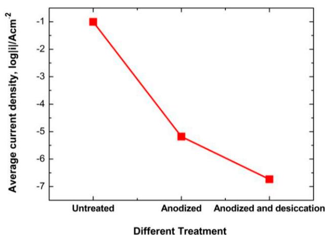
Fig. 8 Average current density between -0.4V and 0V of different treated samples in Fig. 7.
