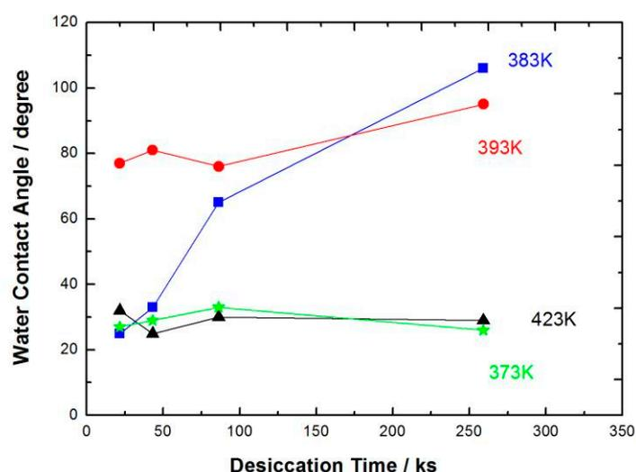
Fig. 3 Water contact angle as a function of time at various desiccation temperature.
