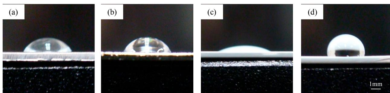
Fig. 1 Side view photographs of water droplet on as-received aluminum (a), as-treated surfaces with electropolishing (b), anodizing (c) and desiccation at 373 K for 1728 ks (d).
