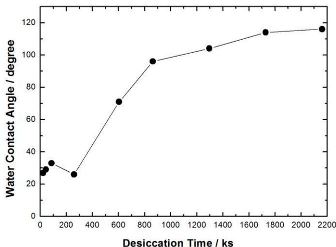
Fig. 4 Change in water contact angle with desiccation time at 373 K.
