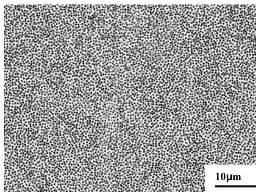
Fig. 6 SEM micrograph of hydrophobic sample after immersed in  $0.6 \text{ kmolm}^{-3}$  NaCl for 3628.8 ks.
