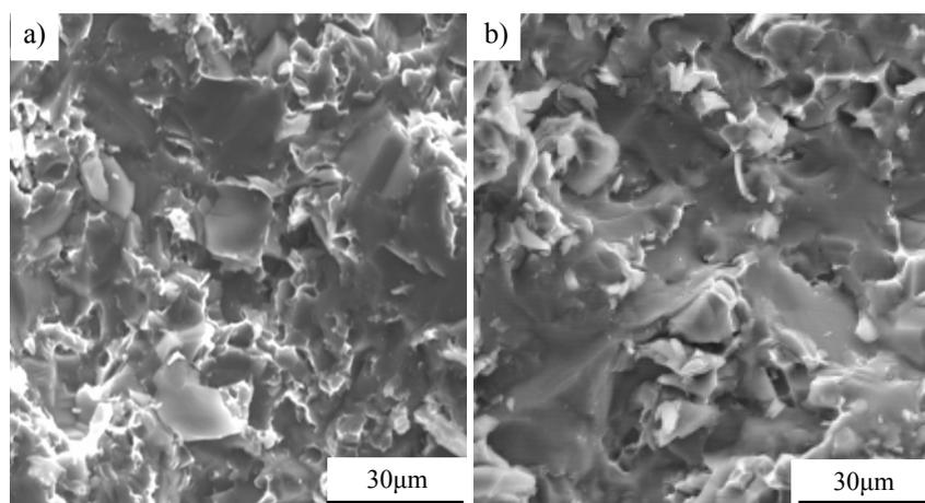
Fig.4 SEM fractographics of Si/1199Al composites
