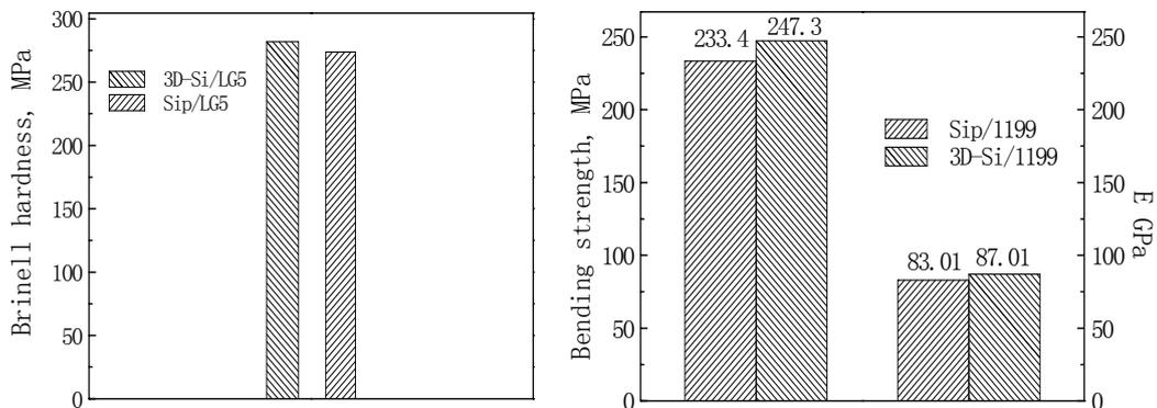
Fig.3 Mechanical properties of Si/1199Al composites
