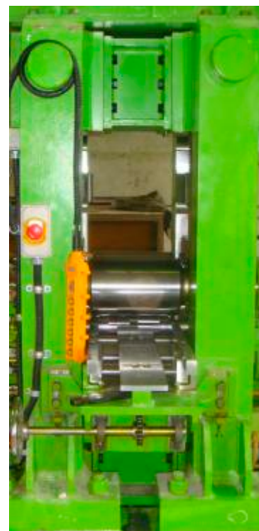
Fig. 3. 6-high roll mill with isothermal internal rollers
