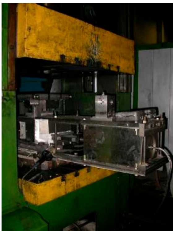
Fig. 2. ECAP die with a back pressure with 400 tons press capacity
