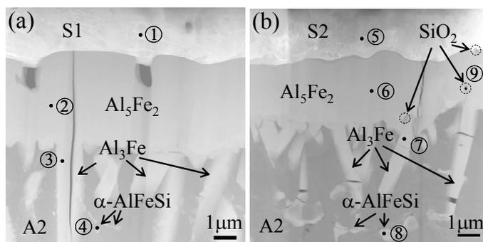
Fig. 5 HAADF-STEM images of IMC layer at the position X in Fig.4: (a) A2/S1, (b) A2/S2.
