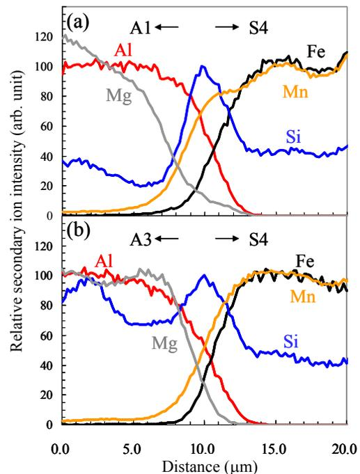
Fig. 9 Composition-depth profile analyzed by SIMS across the IMC layer at the position Y in Fig. 8: (a) A1/S4, (b) A3/S4.
