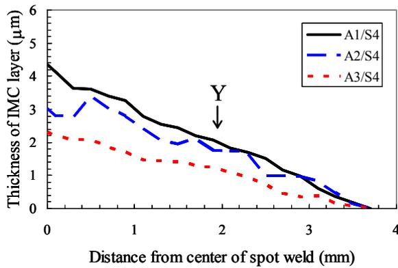
Fig. 8 Effects of Si contents in aluminum alloys on the thickness distribution of IMC layer (30kA, 40ms).
