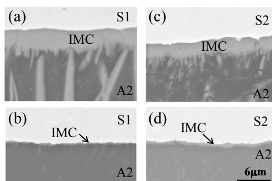
Fig. 3 SEM microstructures of IMC layer formed at the interfaces of steel/ aluminum spot welds (26kA, 40ms): (a) A2/S1, 0.7mm apart in distance from center position in a radial direction, (b) A2/S1, 3.4mm, (c) A2/S2,
