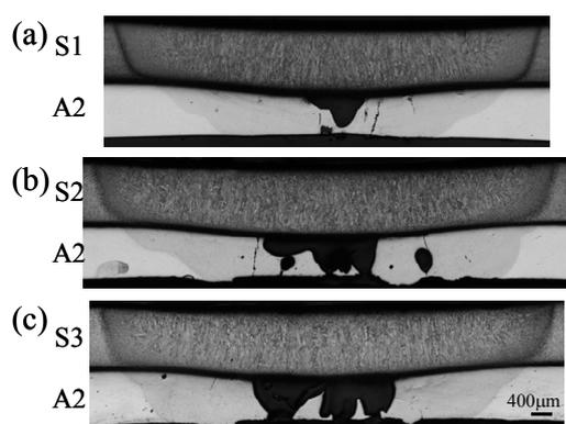
Fig. 2 Macro structures of spot welds (26kA, 40ms): (a) A2/S1, (b) A2/S2, and (c) A2/S3.
