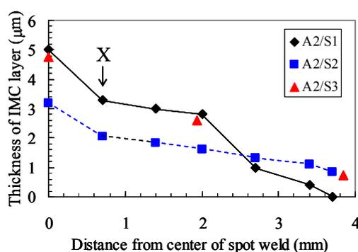
Fig. 4 Effects of Si contents in steels on the thickness distribution of IMC layer (26kA, 40ms).
