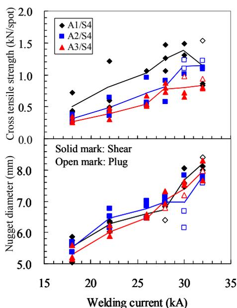
Fig. 6 Variation in the cross tensile strength and nugget diameter with the welding current.
