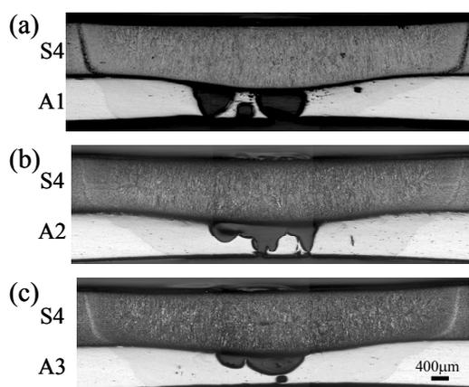
Fig. 7 Macro structures of spot welds (28kA, 40ms): (a) A1/S4, (b) A2/S4, and (c) A3/S4.
