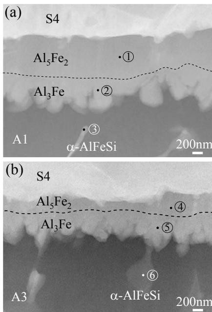
Fig. 10 HAADF-STEM images of IMC layer at the position Y in Fig. 8: (a) A1/S4, (b) A3/S4.
