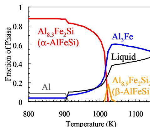
Fig. 11 Equilibrium phase distribution as a function of temperature for the composition of Al-17.6at%Fe-8.8at%Si calculated by Thermo-Calc software.
