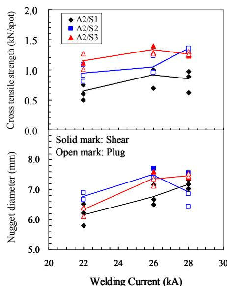
Fig. 1 Variation in the cross tensile strength and nugget diameter with the welding current.
