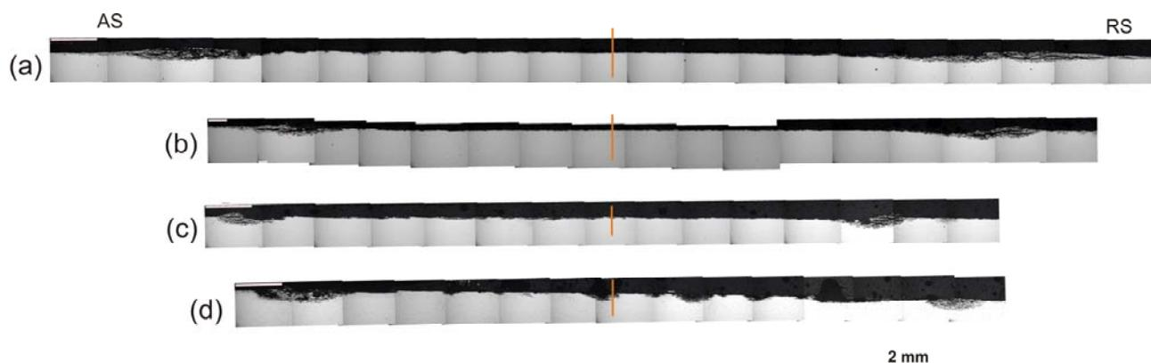
**Fig. 3** Cross transversal sections of FSW 2024-T3 after 24hr immersion in chloride-peroxide solution (a) 100 mm/min, (b) 200 mm/min, (c) 300 mm/min, (d) 400 mm/min
