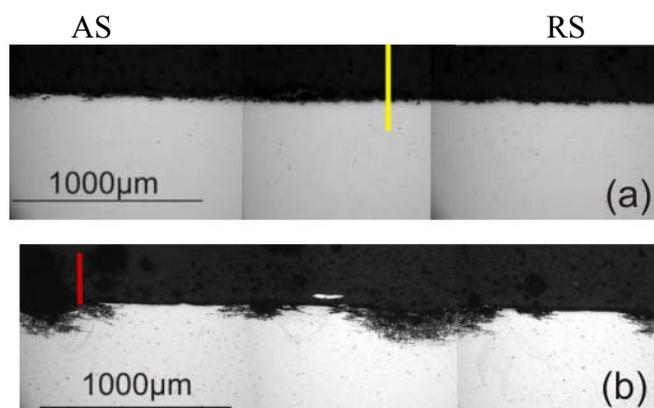
**Fig.4** Effect of welding speed on corrosion behavior of FSW 2024-T3 weld nugget region at the face side (a) 100 mm/min, (b) 400 mm/min
