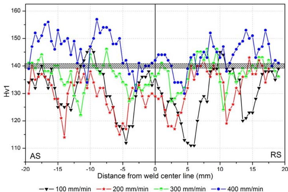
**Fig. 1** Hardness profiles of FSW 2024-T3 joints produced using different welding speeds
