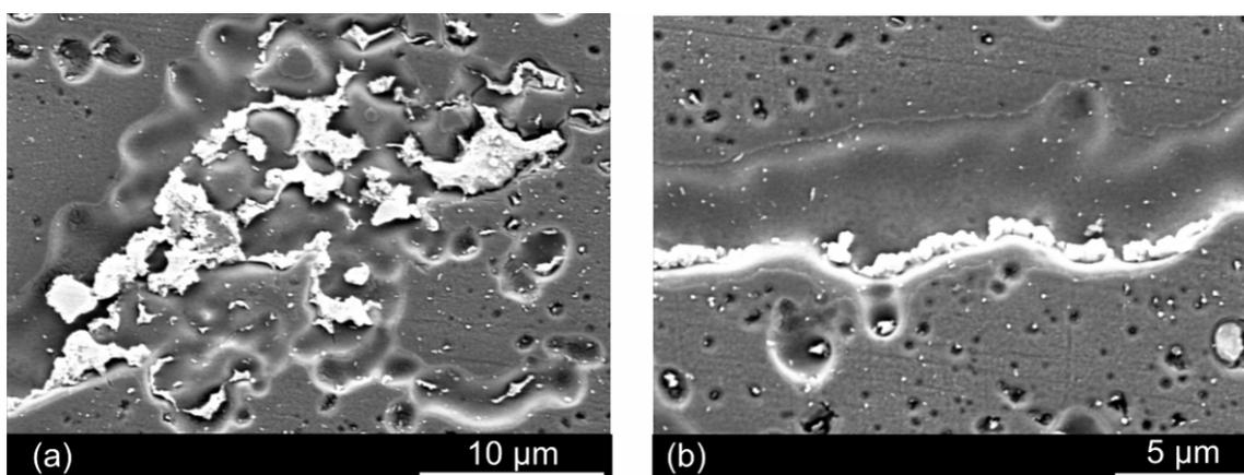
**Fig.6** SEM micrographs of Al–Cu–Mg-containing eutectic phase particles in FSW 2024-T3 joint after 4h exposure to an aqueous 3.5 wt -% NaCl aqueous solution
