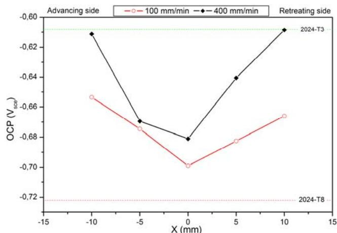
**Fig. 2** Corrosion potential profiles across friction stir welds of alloy 2024-T3 produced with different travel speeds
