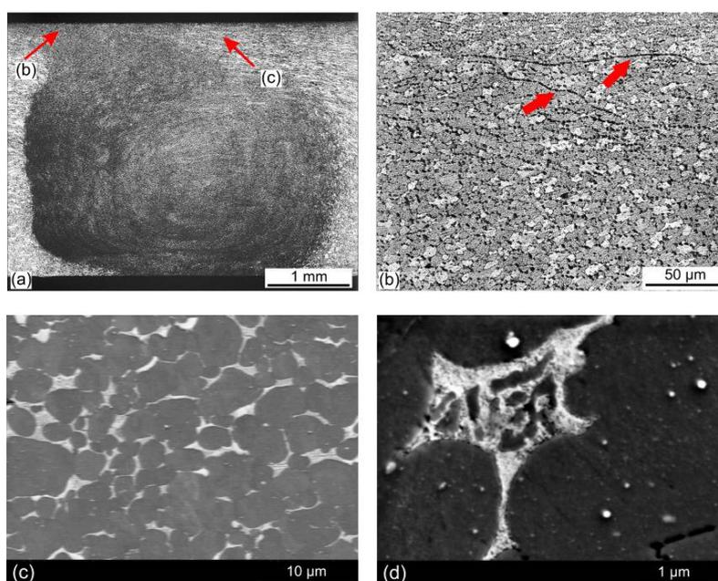
**Fig. 5** Intergranular precipitates found in the flow arm region near to the top surface of the FSW 2024 T3 revealed after etching with Keller's reagent. Arrows in (b-Advancing side) and (c-retreating side) indicate the location of the micrographs.
