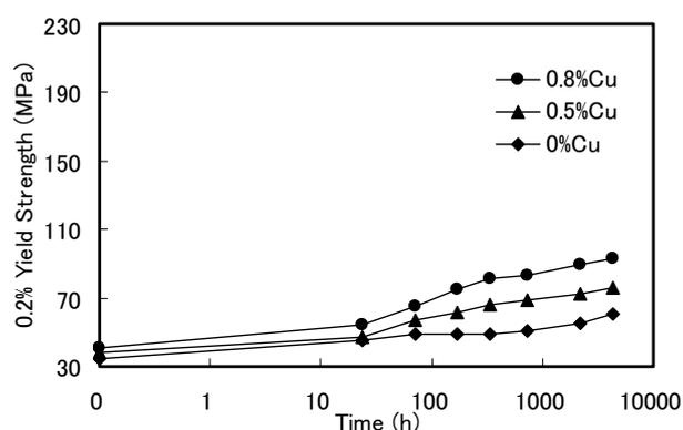
**Fig. 1** Yield strength vs. aging time curves of the alloys aged at RT.
