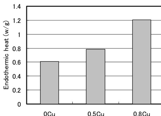
**Fig. 4** The amount of endothermic heat of the alloys aged at RT for 4300h. (Refer to Fig. 3)
