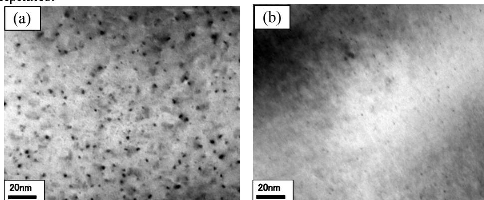
**Fig. 6** TEM images of the 0%Cu alloy-(a) and 0.8%Cu-alloy-(b) aged at 90°C for 720h.
