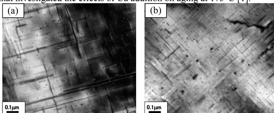
**Fig. 11** Transmission electron micrographs of the 0%Cu alloy-(a) and 0.8%Cu-alloy-(b) aged at 180°C for 170h.
