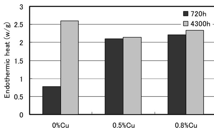
**Fig. 9** The amount of endothermic heat of the alloys aged at 90°C. (Refer to Fig. 8)
