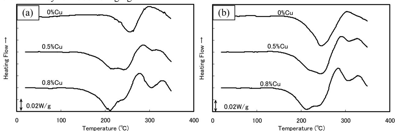
**Fig. 8** DSC curves of the alloys aged for 720h-(a) and 4300h-(b) at 90°C.
