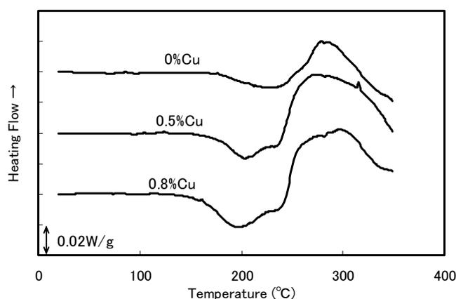
**Fig. 3** DSC curves of the alloys aged at RT for 4300h.
