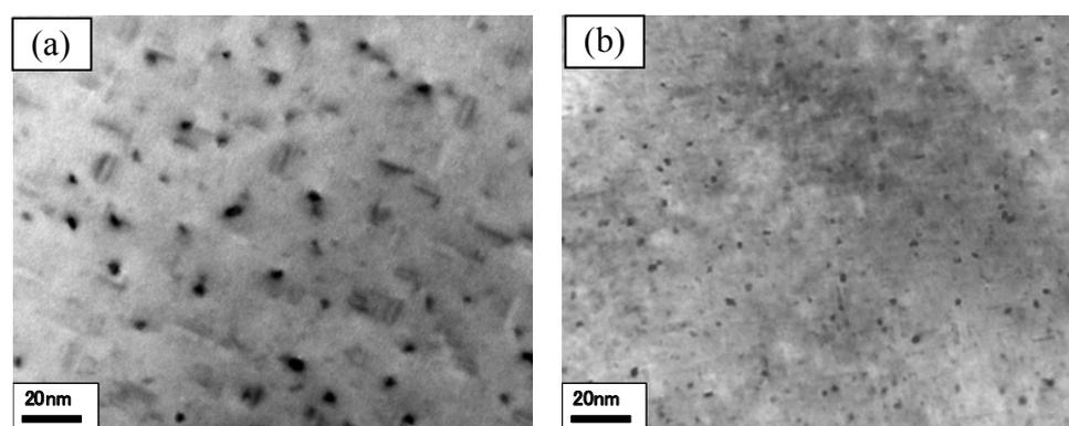
**Fig. 7** TEM images of the 0%Cu alloy-(a) and 0.8%Cu-alloy-(b) aged at 90°C for 4300h.
