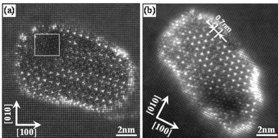
**Fig. 2:** HAADF-STEM image of a  $\beta'$ -phase were observed in the Al-1mass%Mg<sub>2</sub>Si-0.5mass%Ag alloy aged at (a)523K, for 120ks (b)423K, for 12Ms.
