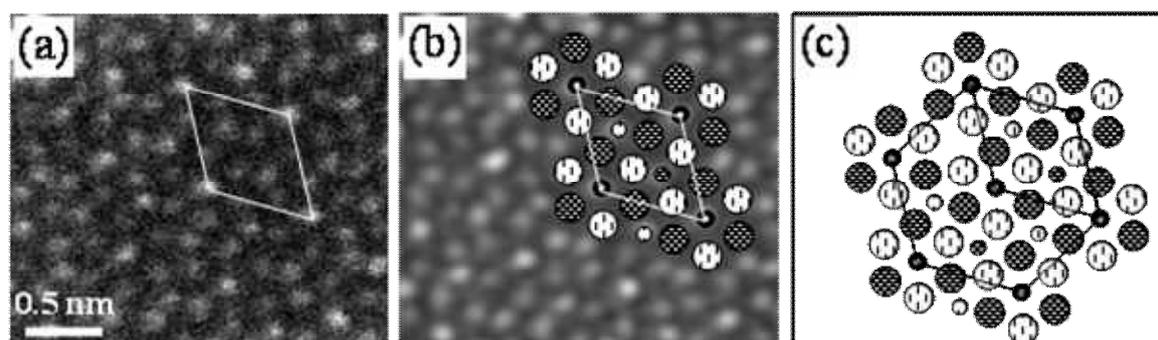
**Fig. 3:** A part of Ag free area in HAADF-STEM image of a  $\beta'$ -phase (a) part of Fig. 2(a), (b) filtered image used by FFT, (c) schematic image of  $\beta'$ -phase without Ag.
