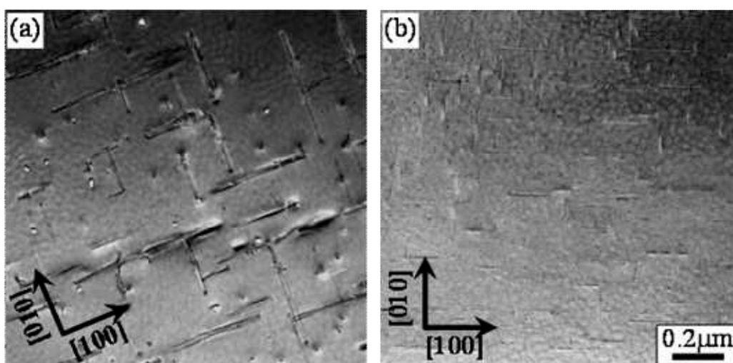
**Fig. 1:** TEM bright field image of the Al-1mass%Mg<sub>2</sub>Si-0.5mass%Ag alloy (a) aged at 523 K for 120 ks, (b) aged at 423 K for 12 Ms.
