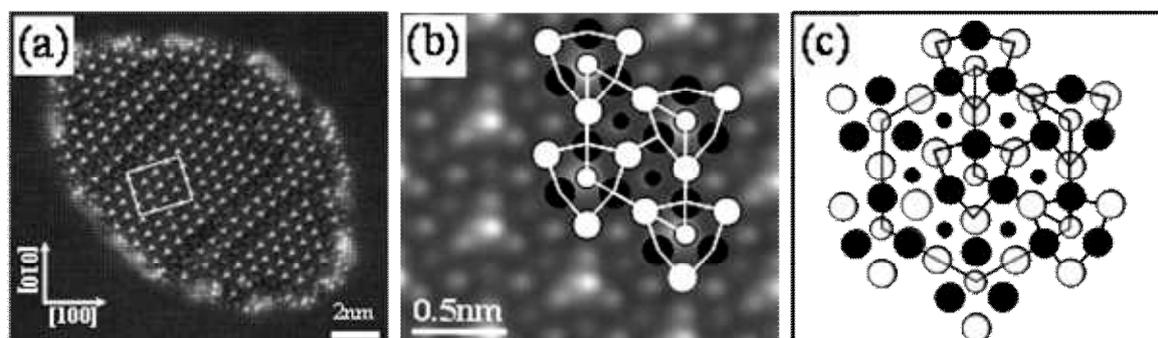
**Fig. 4:** The average image of the parts including Ag observed in a HAADF-STEM image. (a)HAADF-STEM image of the  $\beta'$ -phase, (b) the average image, (c) schematic image of  $\beta'$ -phase with Ag.
