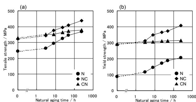
Fig. 4 Effect of natural aging on (a) tensile strength and (b) yield strength of the specimens before artificial aging.
