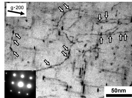
Fig. 9 TEM micrograph of the T8 specimen. The arrows indicate heterogeneous precipitation precipitates on the dislocations.
