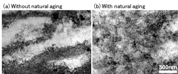
Fig. 7 TEM micrographs of the specimens strained by 20% after solution heat treatment (a) without natural aging and (b) with natural aging at 20°C for 240h.
