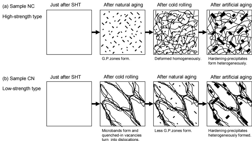
Fig. 10 Schematic diagram of the microstructure in the matrix during the manufacturing processes
