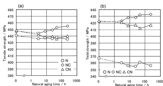
Fig. 5 Effect of natural aging on (a) tensile strength and (b) yield strength of the specimens after artificial aging at 170°C for 8h.
