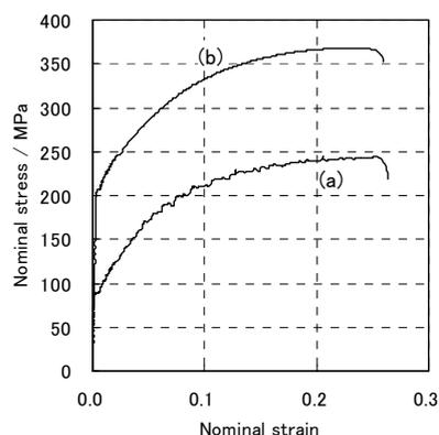
Fig.6 Stress-Strain curve of the specimens after solution heat treatment (a) without natural aging and (b) with natural aging at 20°C for 240h.
