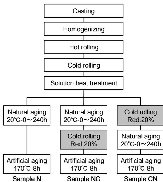
Fig. 1 Flow chart of the manufacturing process.
