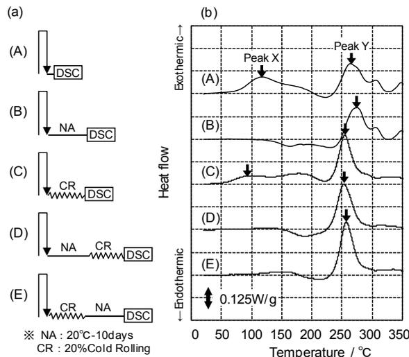
Fig. 8 (a) Schematic diagram of thermomechanical treatments and (b) DSC curves of the specimens subjected to the thermomechanical treatments.
