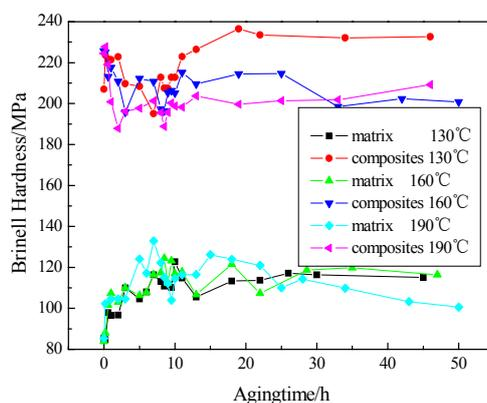
Fig.2 Aging hardening curves of 0.15μm-Al<sub>2</sub>O<sub>3</sub>p/ Al-5.46Cu-Mg composite (Al<sub>2</sub>O<sub>3</sub>p volume fraction: 30%) and matrix alloy at different aging temperatures
