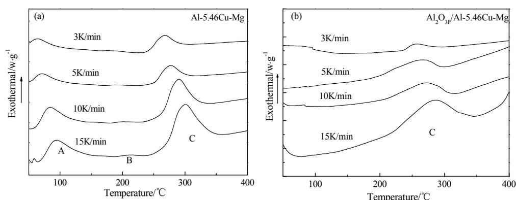
Fig.3 DSC curves at different heating rates for Al-5.46Cu-Mg alloy and the composites treated by solution quenching
