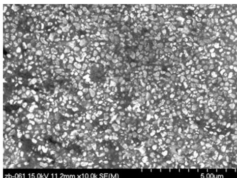
Fig.1 SEM microscopy of the Al<sub>2</sub>O<sub>3</sub>p/Al-5.46Cu-Mg composite
