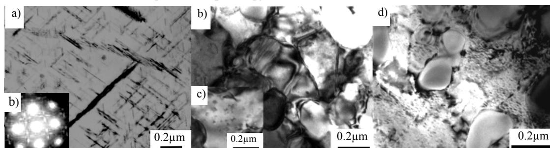
a) Al-5.46Cu-Mg, 190, 25h; b) c)  $\text{Al}_2\text{O}_3\text{p}/\text{Al}-5.46\text{Cu}-\text{Mg}$ , 160, 1h; d)  $\text{Al}_2\text{O}_3\text{p}/\text{Al}-5.46\text{Cu}-\text{Mg}$ , 160, 34h
