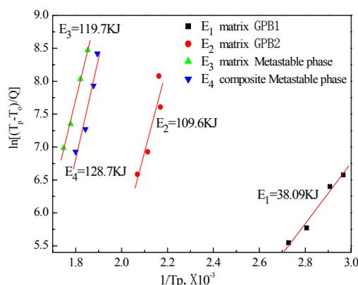
Fig.4 Thermal diffusion activation energy of Al<sub>2</sub>O<sub>3p</sub>/ Al-5.46Cu-Mg composites and the matrix alloy
