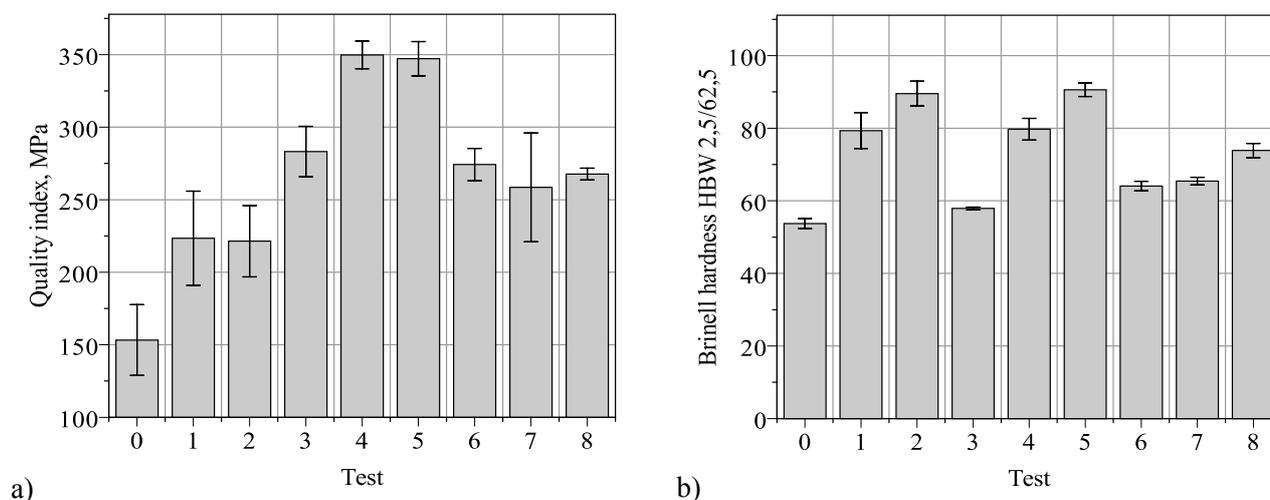
Fig. 4: a) Q-Index and b) Brinell hardness from the individual tests.
