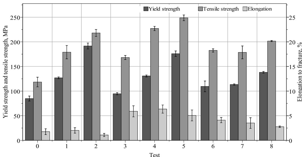
Fig. 3: Yield strength, tensile strength and elongation from the individual tests.
