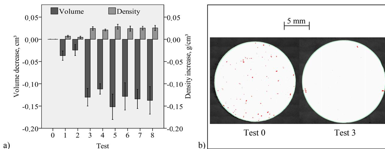
Fig. 2: a) Volume decrease and density increase depending on the treatment conditions; b) Porosity (marked red) after the treatment for test 0 and 3.
