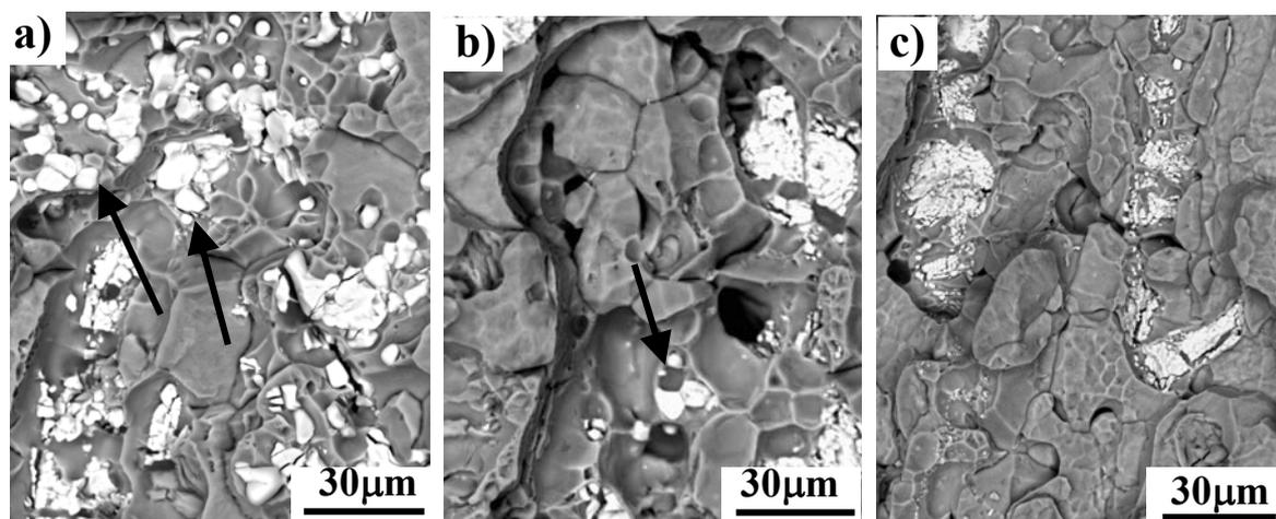
Fig. 4. Fractographs of: a) 475°C-, b) 485°C- and c) 495°C-optimised samples after RRA treatment as indicated in Table 1. Images were taken using backscattered electron imaging and particles were identified by EDS. Arrows point to S-phase particles, none of which could be found in image (c). Other bright particles are  $Al_7Cu_2Fe$ .
