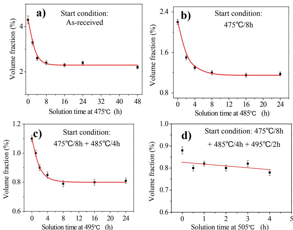
Fig. 1. Volume fraction changes of remaining constituent particles in differently solution treated samples: a) 475°C for different times, b) 475°C/8h + 485°C for different times, c) 475°C/8h + 485°C/4h + 495°C for different times and d) 475°C/8h + 485°C/4h + 495°C/2h + 505°C for different times.
