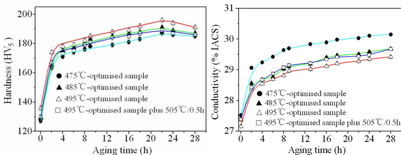
Fig. 3. Hardness and electrical conductivity responses of the differently solution-treated samples during artificial ageing at 120°C.
