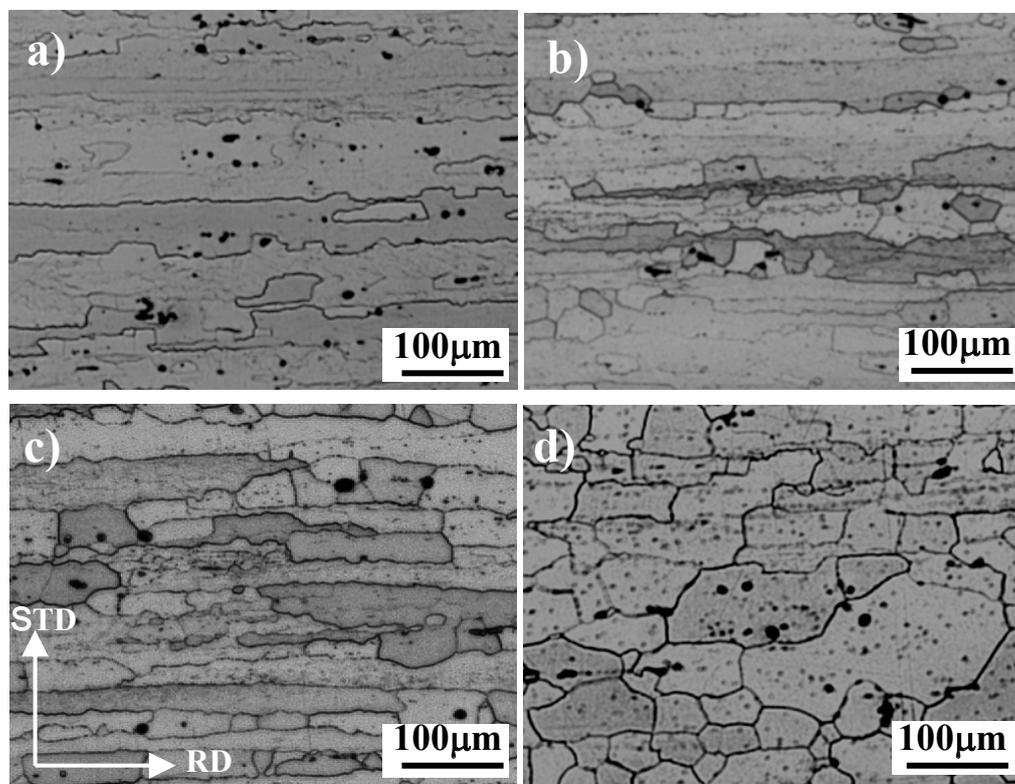
Fig. 2. Optical micrographs of typical grain structures from differently solution-treated samples: a)  $475^{\circ}\text{C}/8\text{h}$ , b)  $475^{\circ}\text{C}/8\text{h} + 485^{\circ}\text{C}/4\text{h}$ , c)  $475^{\circ}\text{C}/8\text{h} + 485^{\circ}\text{C}/4\text{h} + 495^{\circ}\text{C}/2\text{h}$  and d)  $475^{\circ}\text{C}/8\text{h} + 485^{\circ}\text{C}/4\text{h} + 495^{\circ}\text{C}/2\text{h} + 505^{\circ}\text{C}/0.5\text{h}$ .
