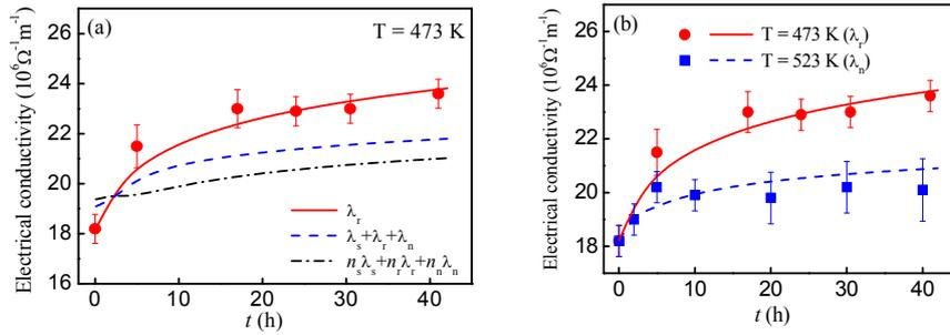
Fig. 3 Experimental and calculated dependence of the electrical conductivity ( $\kappa$ ) on  $t$  at  $T = 473$  K and  $523$  K. Dots are experimental results and lines are calculations. In (a), calculations are based on Case I (Eq. 4), Case II (Eq. 5), and Case III (Eq. 6). Calculations fitting well with the experiments at both the two aging temperature are summarized in (b).
