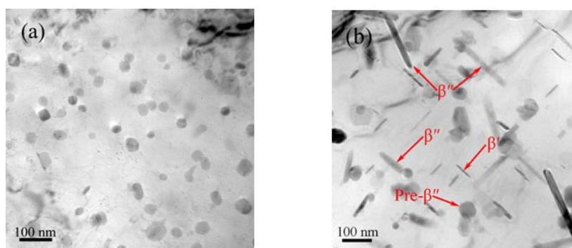
Fig. 1 Typical TEM images showing the morphology and size of pre- $\beta''$  precipitates of  $\text{AlMg}_4\text{Si}_6$  before secondary aging treatment (a) and of multiple precipitates, i.e., sphere-shaped pre- $\beta''$  particles of  $\text{AlMg}_4\text{Si}_6$ , rod-shaped  $\beta''$  precipitates of  $\text{Mg}_5\text{Si}_6$ , and needle-shaped  $\beta'$  precipitates of  $\text{Mg}_2\text{Si}$ , after secondary aging treatment.
