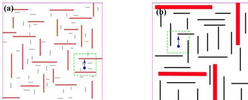
Fig. 4 Sketches illustrating the rod-shaped  $\beta''$  and needle-shaped  $\beta'$  precipitates forming the dominant effective hindrance net to mass migration in (a)  $T = 473$  K, and (b)  $T = 523$  K, respectively.
