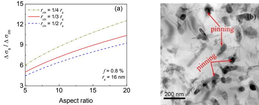
Fig. 2 (a) Dependence of  $\Delta\sigma_s / \Delta\sigma_{r/d}$  on rod-/needle-shaped precipitate size ( $r_{r/d}$ ) as a function of the aspect ratio of the rod-/needle-shaped precipitates; (b) Typical TEM image showing the pinning of dislocations by spherical precipitates.
