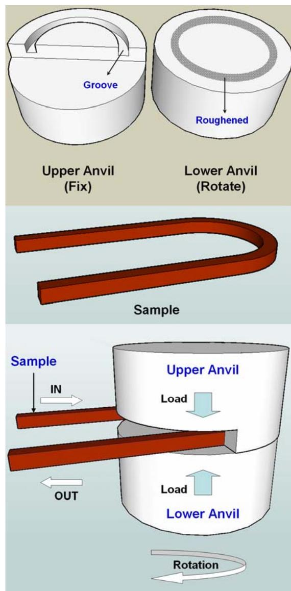
Fig. 1. Schematic illustration of CHPT.
