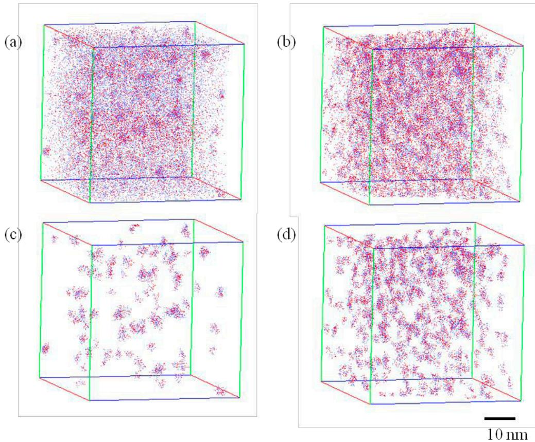
Fig.4 Mg and Si atom map in B alloy aged at 373 K for 120 h (a) and the one in ES alloy aged at 373 K for 600 h (b) obtained in 3DAP measurement and Mg and Si map after particle analysis in B alloy (c) and the one in ES alloy (d); in (a) and (b) the dense regions in both alloys indicate the Mg-Si clusters, while the other regions indicate the Mg and Si atoms as solid solution. The Mg and Si atoms are depicted by blue and red, respectively.
