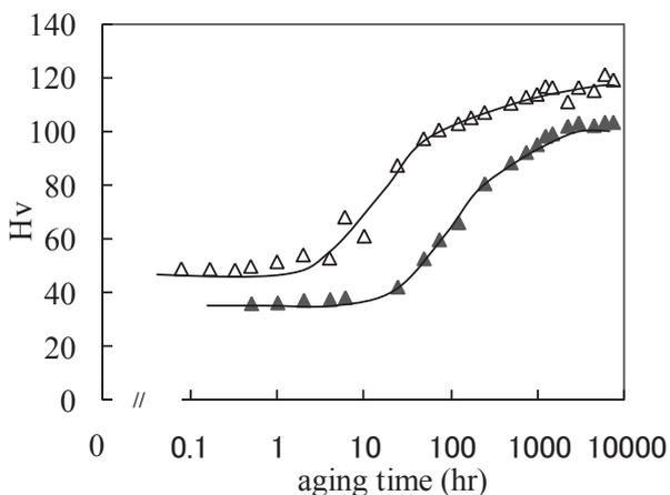
Fig.2 The aging curve of Vickers hardness;
