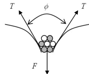
Fig.1 Dislocation-precipitate interaction
