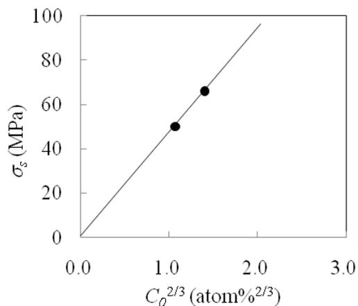
Fig.5 Relationship between the concentration of Mg and Si atoms,  $c_0$  and the yield strength induced by these atoms,  $\sigma_s$ . Both values is obtained in the tensile tests in alloy B and alloy ES as quench. An inclination is estimated at 38.98.
