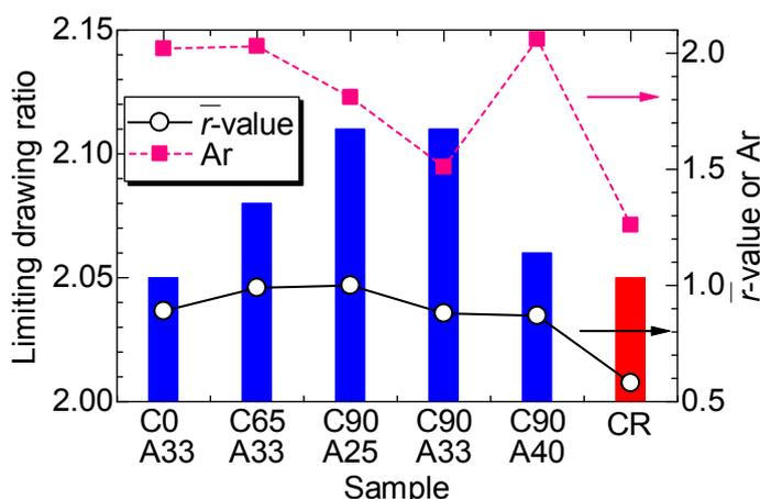
Fig. 7 Effect of  $r$ -value on limiting drawing ratio for samples produced by various rolling processes.  $Ar$  is the anisotropic parameter defined by  $Ar = r_{\max}/r_{\min}$ .
