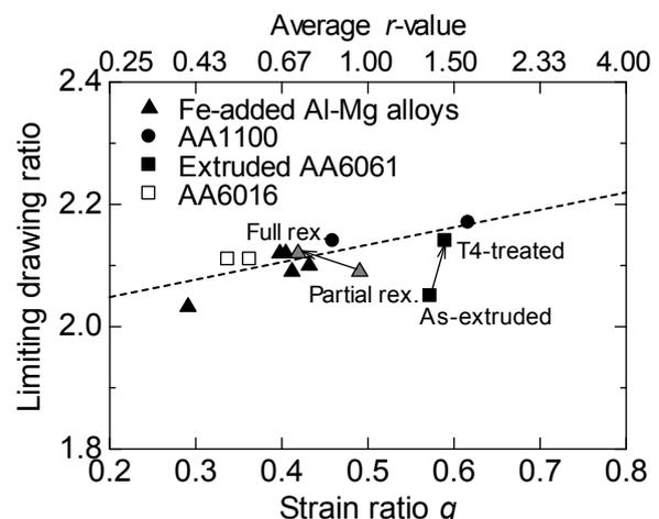
Fig. 1 Correlation between average  $r$ -value and LDR for aluminum alloys with various textures.
