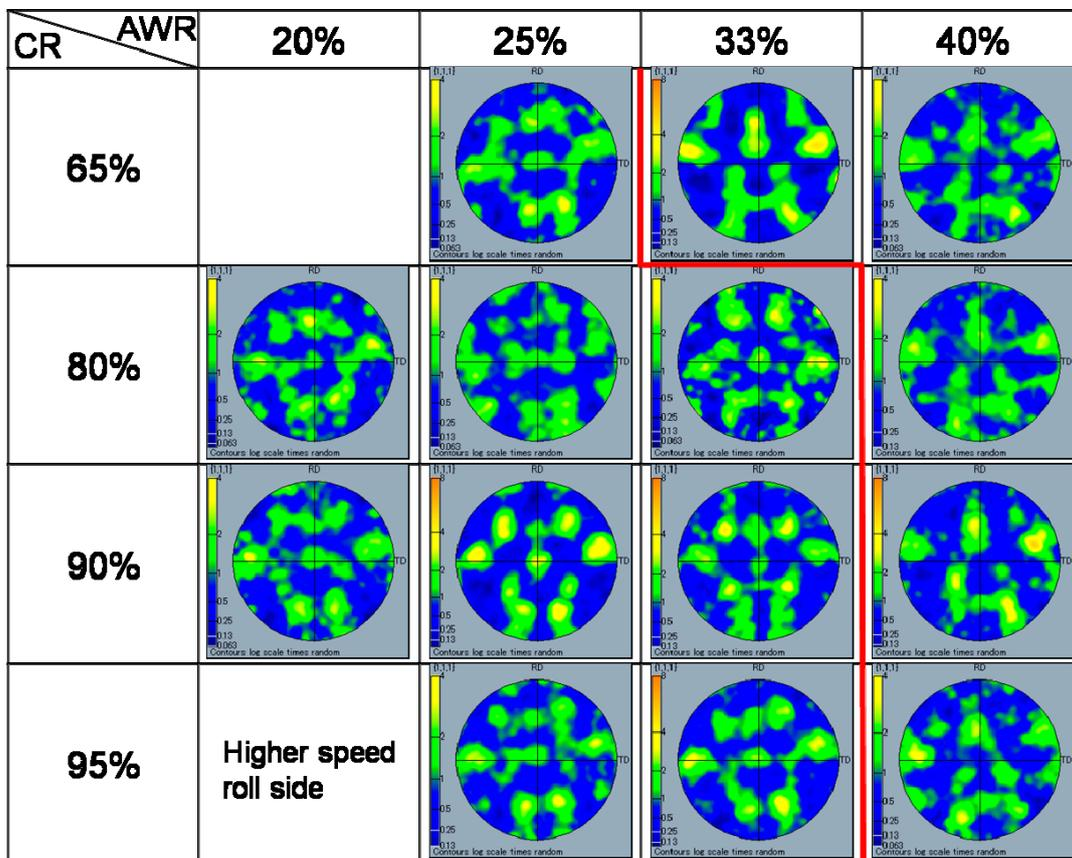
Fig. 5  $\{111\}$  pole figures of recrystallization textures measured on the longitudinal section by the SEM-EBSD method for AA6022 alloy sheets solution-treated at 813 K for 90 s after cold rolling (CR) and subsequent asymmetric warm rolling (AWR).
