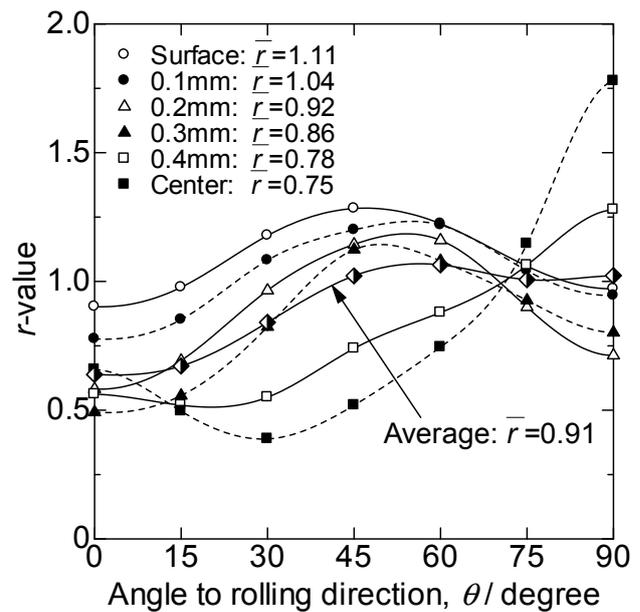
Fig. 4 Planar anisotropy of  $r$ -value at different locations calculated by the RC model from the texture at each layer for warm rolled and annealed Al-4.3%Mg-0.3%Fe alloy sheet.
