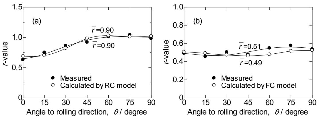
Fig. 3 Comparison between measured and calculated  $r$ -values for (a) Al-4.3%Mg-0.3%Fe and (b) AA6016 alloy sheets with recrystallization textures shown in Fig. 2.
