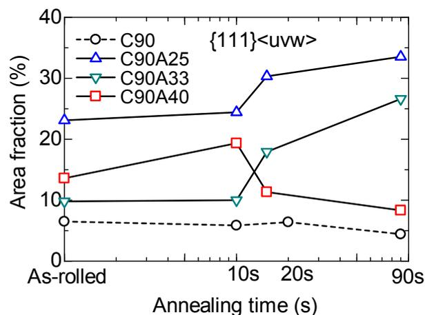
Fig. 6 Change in area fraction of  $\{111\}\langle uvw\rangle$  component during annealing at 813 K for 90% cold rolled samples. Here C90A25 means a sample produced by the process of 90% cold rolling + 25% asymmetric warm rolling.
