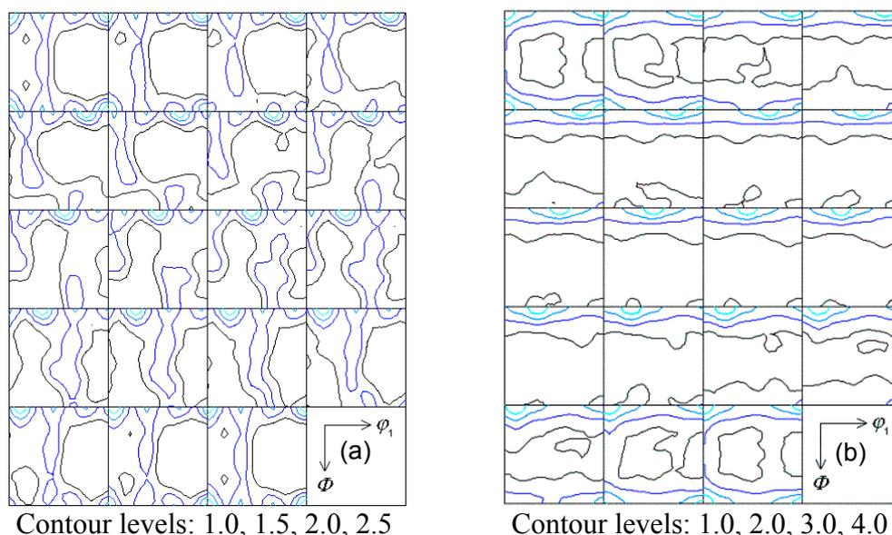
Fig. 2 Overall textures through sheet thickness for (a) Al-4.3%Mg-0.3%Fe alloy sheet annealed at 573 K for 10 ks and (b) AA6016 alloy sheet solution-treated at 793 K for 960 s after warm rolling to about 90% reduction.
