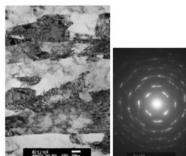
**Figure 5** TEM micrographs of ASRed sample at equivalent strain of 154%
