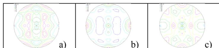
With respect to the starting material, featuring a fully annealed texture (Figure 3), after the first four rolling steps, a very weak brass texture is still present, even if the values of relative intensity are very low as shown in Table 1.
