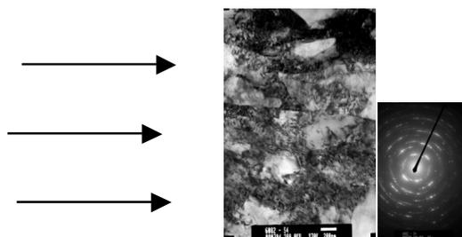
**Figure 4** TEM Micrograph of ASRed sample subjected to equivalent strain of 77% and correspondent SADP
