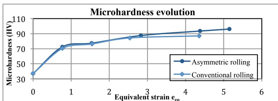
Figure 1 Evolution of microhardness as a function of equivalent strain
