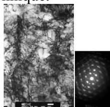
Figure 6 TEM Micrograph of ASRed sample at equivalent strain of 515%
