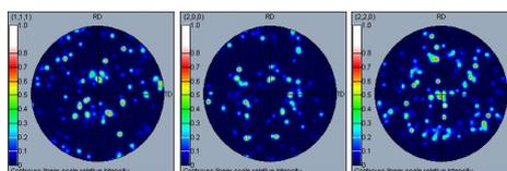
Figure 3 Pole figures of the annealed starting material
