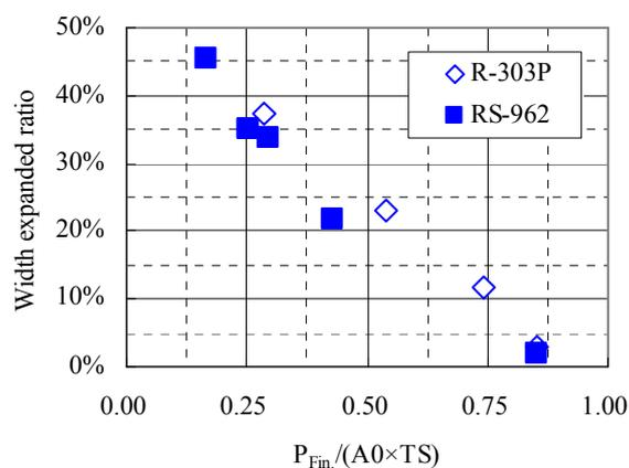
Fig. 9. Relationship between punch load at the end and the width expanded ratio
