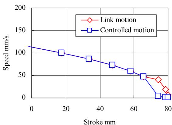
Fig. 6. Speed diagrams of slide motion
