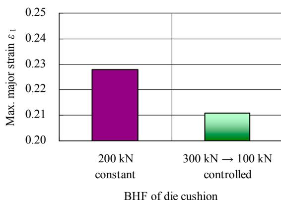
Fig. 4. Maximum major strain  $\varepsilon_1$  at the punch shoulder in the case of Controlled motion
