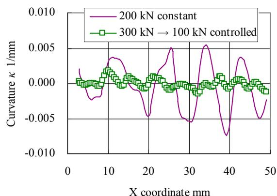
Fig. 5. Curvature distribution of measured line at the flange in the case of Controlled motion
