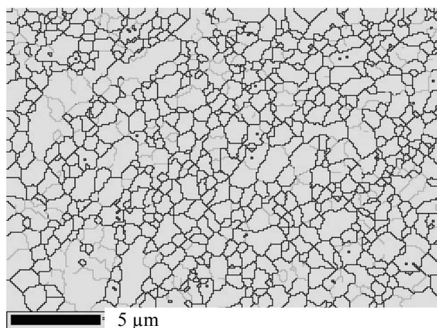
Fig. 3 EBSD analysis of Al-1050 alloys processed by twelve passes of ECAP
