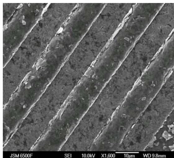
Fig. 6 SEM secondary electron images showing the topography of hot embossed UFG Al-1050 produced by four passes of ECAP. Channels are  $10\mu\text{m}$  wide and  $10\mu\text{m}$  deep.
