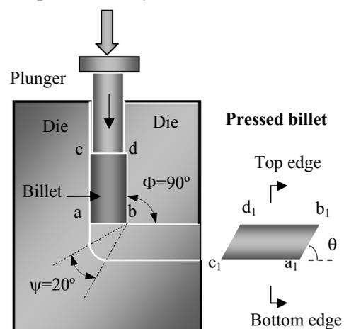
Fig. 1 Facility and principle of ECAP
