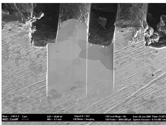
Fig. 7 FIB secondary electron image of cross section of hot embossed UFG Al-1050 produced by eight passes of ECAP.
