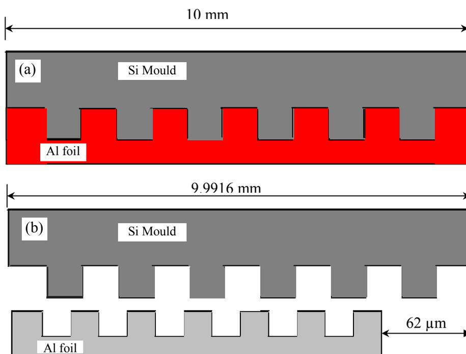
Fig. 8 Schematically illustration of thermal expansion of an Al foil and a Si mould during hot embossing and demoulding. (a) Embossing at 300 °C, (b) Demoulding at room temperature.
