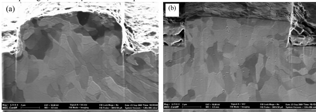
Fig. 5 FIB images of the cross section of the cold embossed Al-1050 foils processed by various passes of ECAP, a) two passes; b) eight passes.
