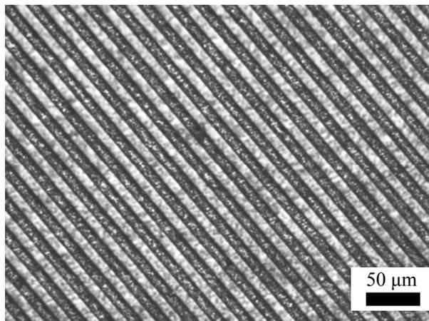
Fig. 4 Optical micrograph of the embossed topography of the UFG Al-1050 foil after two passes of ECAP.
