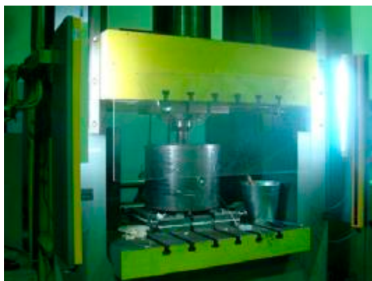
Fig. 1. LHIP vessel with 400 tons press capacity
