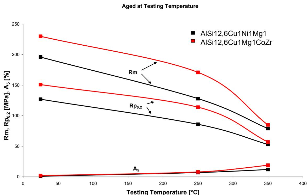
**Fig. 1:** Mechanical properties of tested alloys as a function of temperature
