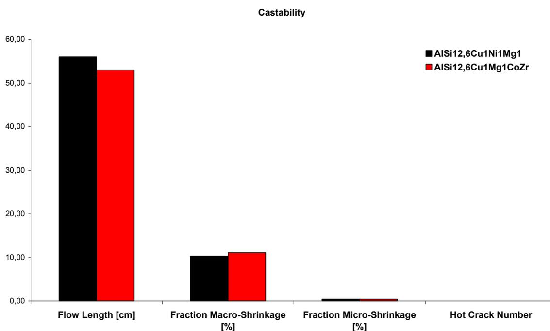
**Fig. 2:** Castability of tested alloys
