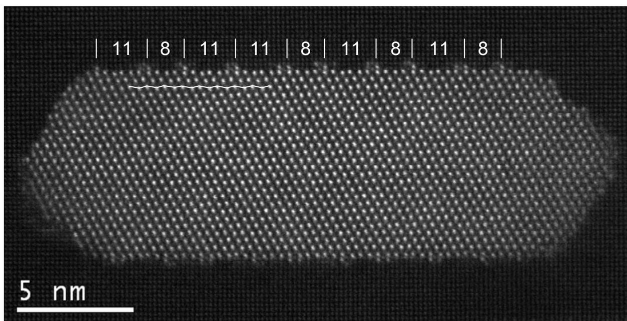
**Fig. 2:** Unprocessed HAADF STEM image of a U1-like precipitate from the same condition. The zigzag line formed by the Ge columns at the interface is not as uniform as that in the bulk of the precipitate (shown). The vertical lines indicate the extra Ge columns where the zigzag line points into the precipitate. The numbers indicate the number of  $(200)_{\text{Al}}$  planes between the lines.
