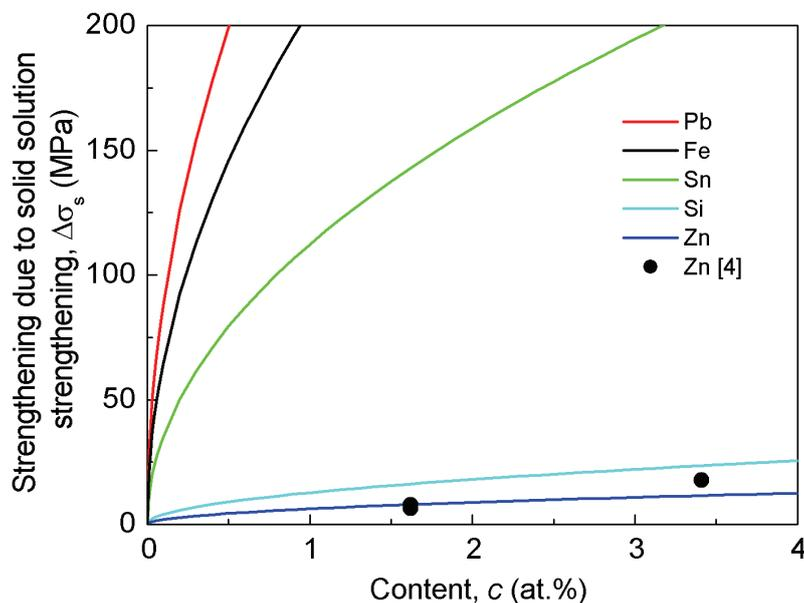
Fig. 2 The dependence of the contribution to the yield stress due to the solid solution strengthening as a function of the solute content in Al-Si, Al-Zn, Al-Sn, Al-Pb and Al-Fe alloys. Filled circles are the experimental results of Al-Zn alloys [4].
