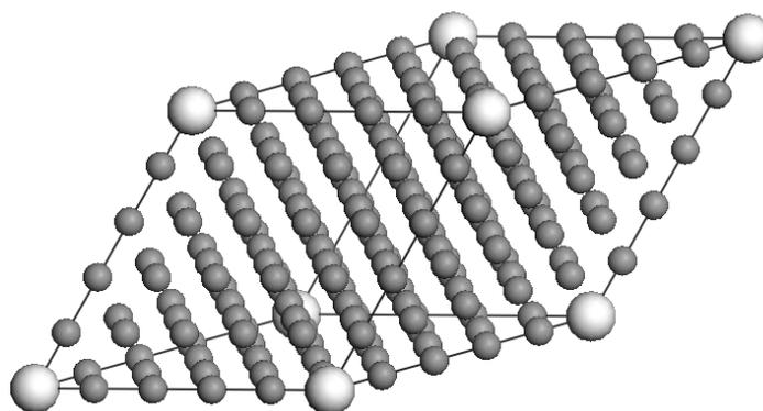
Fig. 1 Depiction of supercell containing 124 Al atoms and one solute atom for the calculations of misfit strains in Al-based solid solutions. Gray balls indicate Al atoms and white balls indicate solute atoms.
