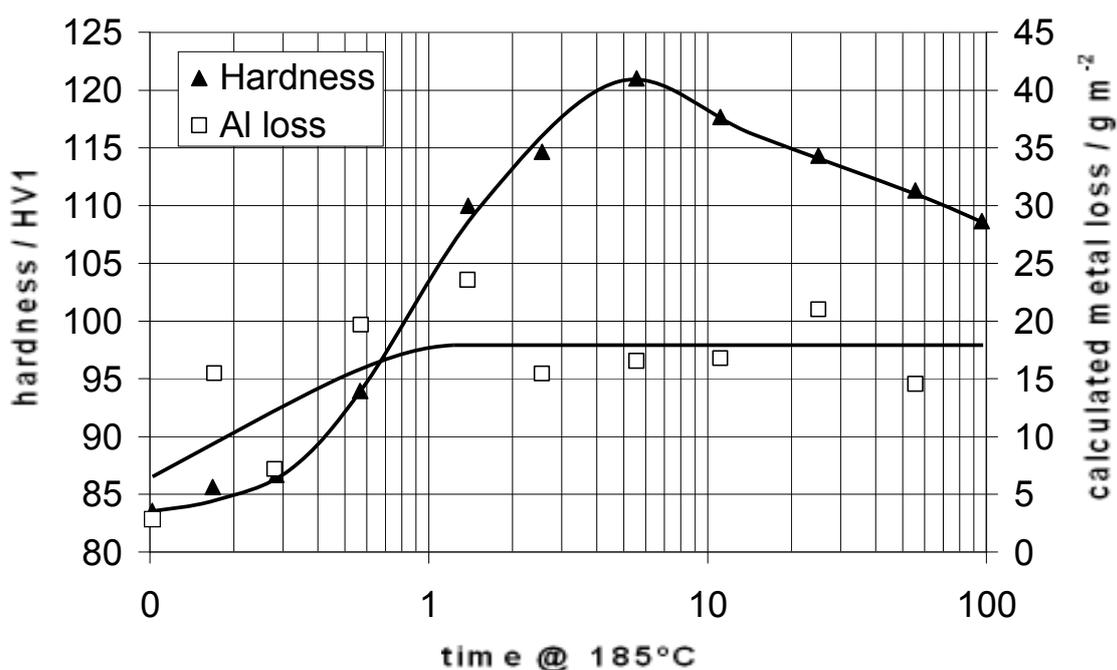
Fig. 3.1 Hardness and calculated metal loss of AA6111 samples heat treated for times up to 96h.
