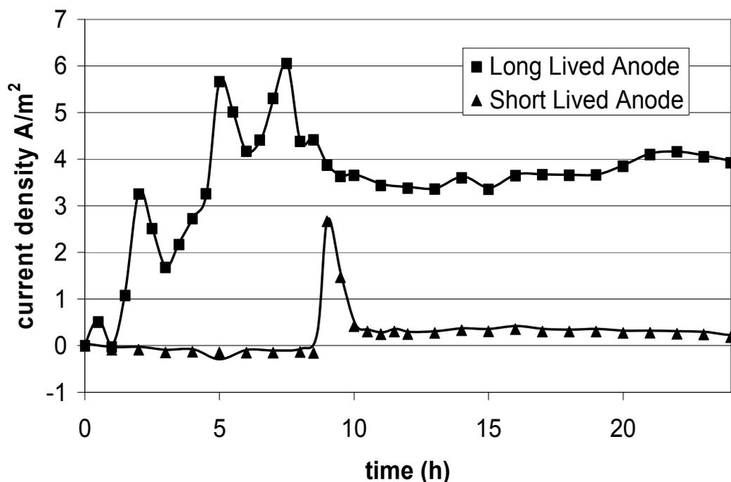
**Fig. 3.4** SVET current density profiles of two anodes on peak aged (5.56h @ 185°C) AA6111 during 24h immersion in 1% w/w aqueous NaCl solution.
