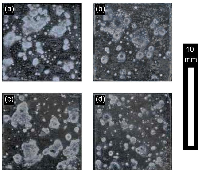
**Fig. 3.2** Photographs of 10mm by 10mm exposed area of samples in the T4 (0h @ 185°C), underaged (0.57h @ 185°C), peak aged (5.56h @ 185°C) and overaged (55.56h @ 185°C) conditions after 24h immersion in 1% w/w aqueous NaCl solution.
