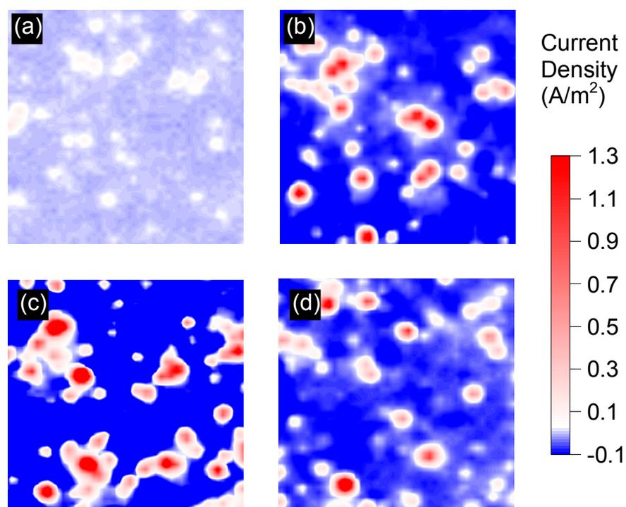
**Fig. 3.3** SVET current density maps of 10mm by 10mm exposed area of samples in the T4 (0h @ 185°C), underaged (0.57h @ 185°C), peak aged (5.56h @ 185°C) and overaged (55.56h @ 185°C) conditions after 24h immersion in 1% w/w aqueous NaCl solution.
