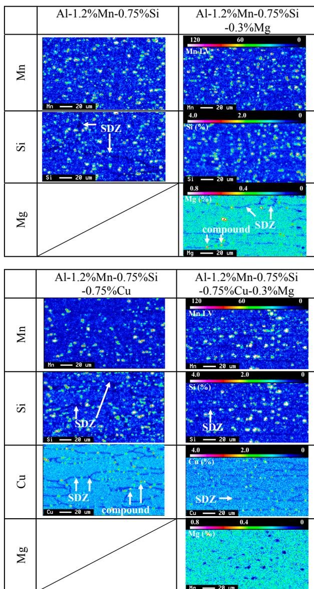
**Fig.5** EPMA analysis after heating for 100h at 473K.
