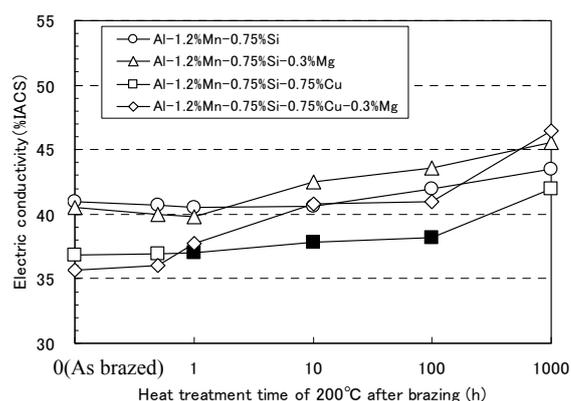
**Fig.4** Variation of electric conductivity with heating time.
