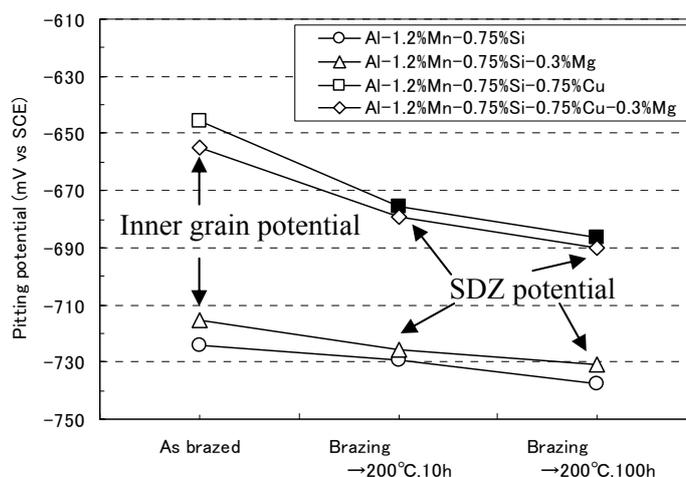
**Fig.9** Variation of pitting potential on materials with heat treatment.
