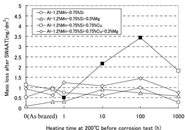
**Fig.3** Mass loss and corrosion form after SWAAT 72h.
