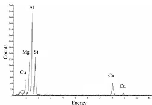
**Fig.7** Example of EDS analysis result of needle shape compound.
