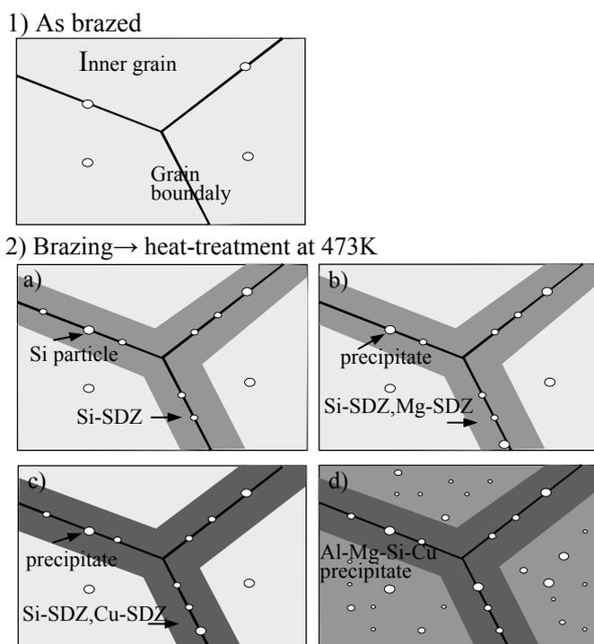
**Fig.8** Schematic representation of metallurgical structure around grain boundary.
