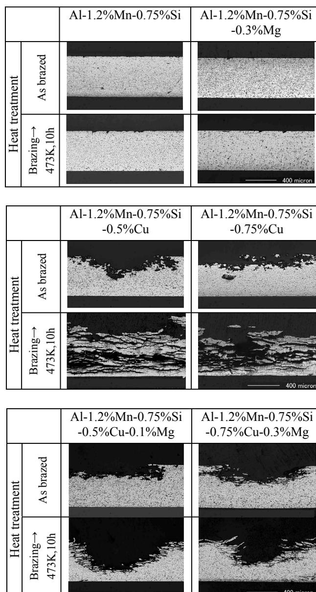
**Fig.2** Cross section observation of localized corrosion after SWAAT 72h.
