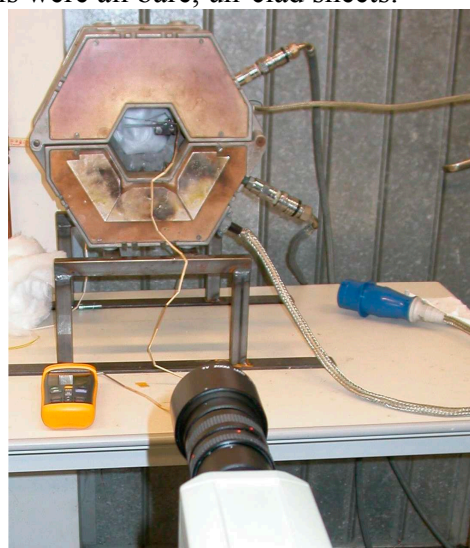
Fig.1(b) Equipment for continuous monitoring of sagging during a heating cycle
