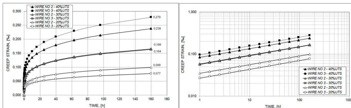
Fig.4. Creep profiles of AlMgSi wires (2 and 3) obtained in temperature 20°C and under stress 20, 30, and 40% UTS, during 160 h of the process.
