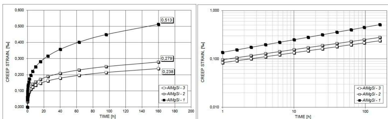
Fig.3. Creep profiles of AlMgSi wires obtained in temperature 20°C and under stress 40% UTS, during 160 h of the process.
