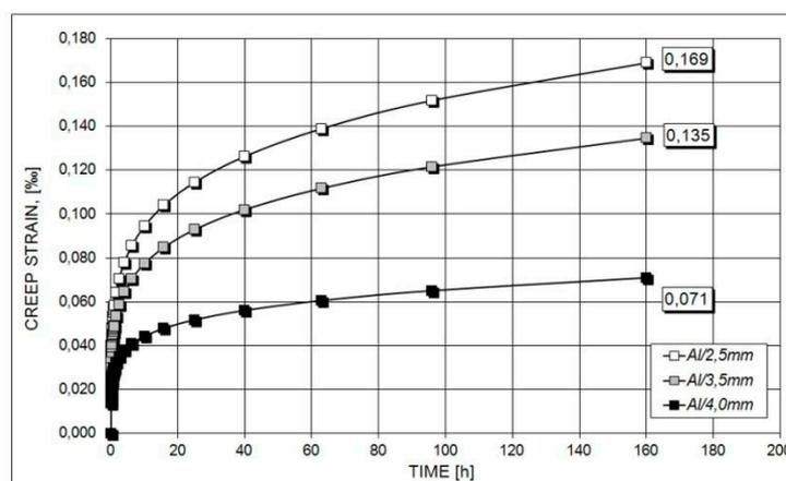
Fig.2. Creep characteristics of aluminium wires, creep conditions: temperature– 20°C, stress – 20% UTS, time – 160 h (comp. Tab. 1).
