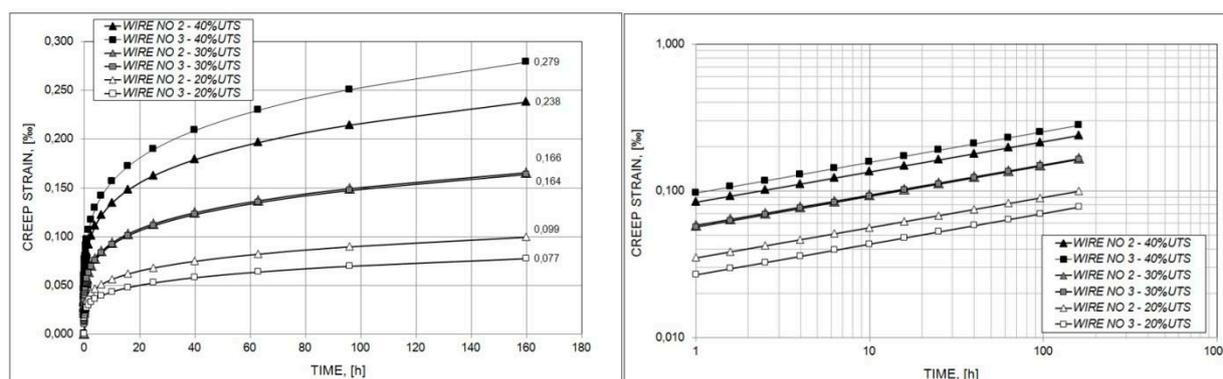
Fig.4. Creep profiles of AlMgSi wires (2 and 3) obtained in temperature 20°C and under stress 20, 30, and 40% UTS, during 160 h of the process.
