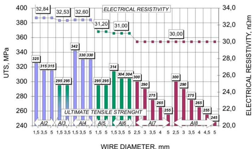
Fig. 1 Minimum tensile strengths and permissible resistivity of AlMgSi wires according to EN 50183:2000 [1]
