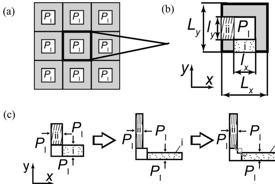
Fig. 1 Schematic illustration of the 2D-square model for solid-state foaming. The infinite body placed the square pores systematically (a), (b) the unit-square cell on the infinite body and (c) the deformation process of the elements  $i$  and  $ii$  in (b).
