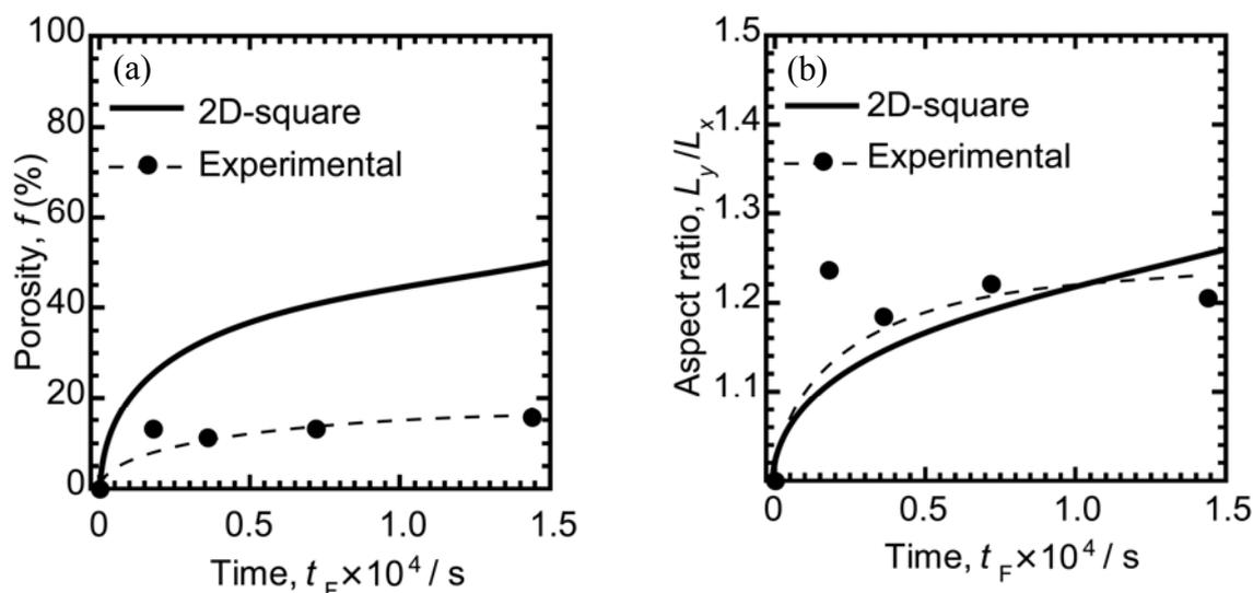
Fig. 3 Comparison of the model analysis with experimental results. The time dependency (a) of the porosity and (b) of the foam aspect ratio.
