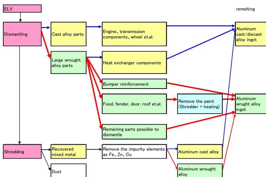
Fig.7 Recommended aluminum material recycling flow by ELV
