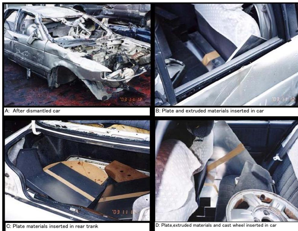
Fig.4 Appearance of the inserted materials at the shredding test
