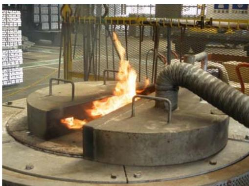
Fig.6 Appearance of the melting furnace without any pre-treatment
