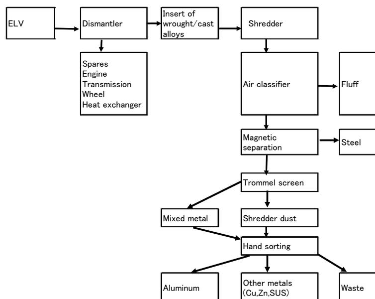
Fig.3 Flow of the shredding test
