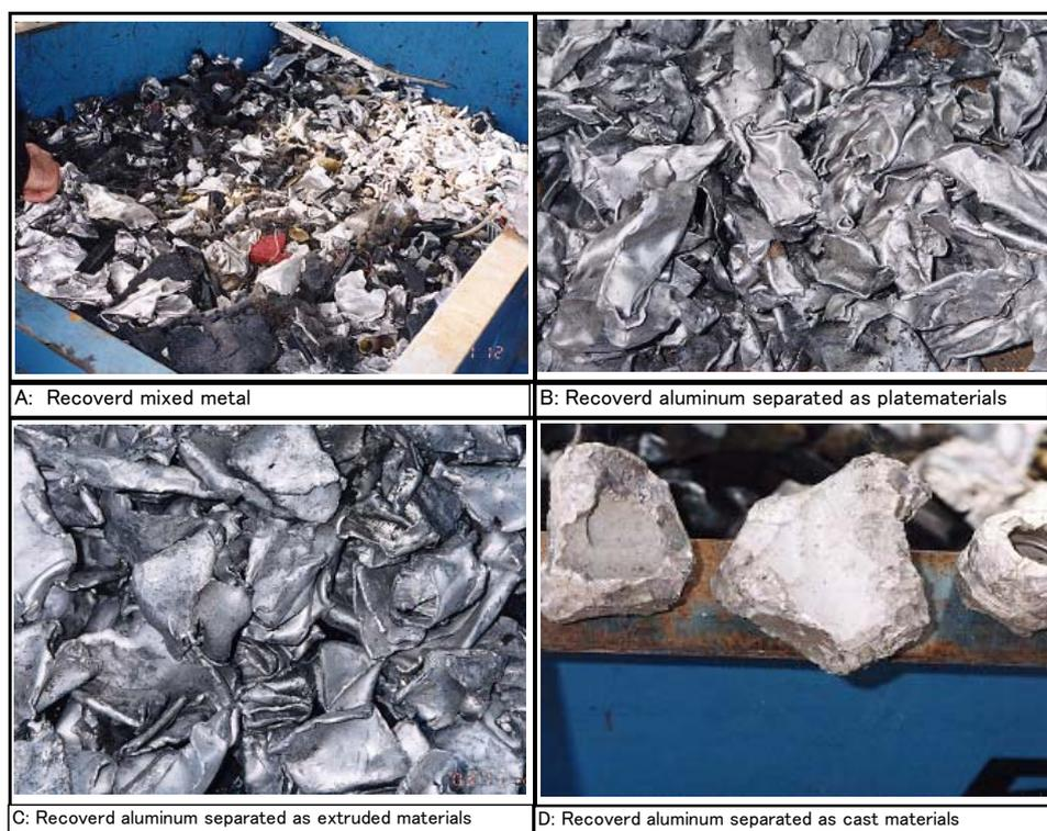
Fig.5 Appearance of the recovered aluminum alloy materials
