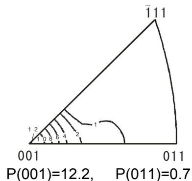
Fig. 5 Development of  $\{001\}$  fiber texture in Al-4.6Cu by the deformation at  $803\text{K}$  with a strain rate of  $5.0 \times 10^{-3} \text{s}^{-1}$  up to a strain of  $-1.0$ .
