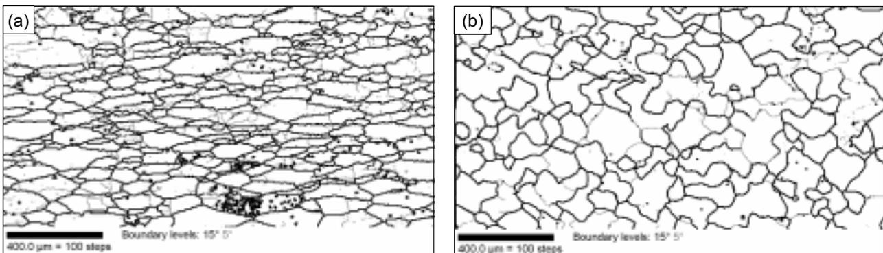
Fig. 7 Microstructures observed at the cross section after the deformation at 723K with a strain rate of  $5.0 \times 10^{-4} \text{ s}^{-1}$  up to -1.0 in true strain. (a) Al-3Mg-0.2Sc and (b) Al-10Mg. Thick and thin lines express the high angle grain boundaries with the misorientations higher than 15 degrees and low angle grain boundaries, respectively.
