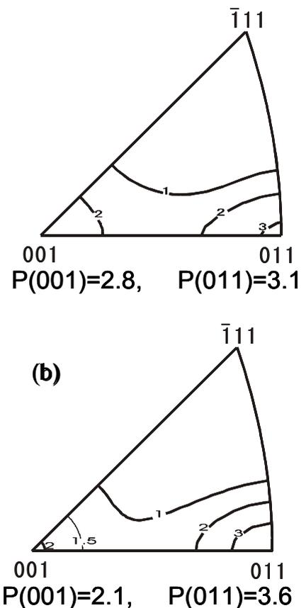
Fig. 6 Inverse pole figures for the compression plane after the deformation at 723K up to a strain of -1.0. (a) Al-3Mg and (b) Al-3Mg-0.2Sc [2].
