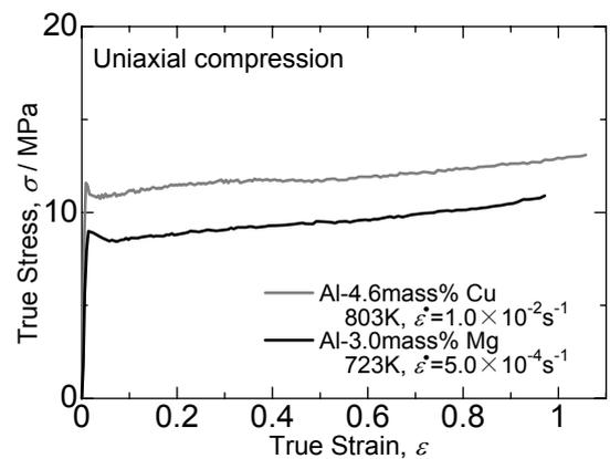
Fig. 1 True stress-true strain curves of Al-3Mg and Al-4.6Cu alloys. Deformation conditions for Al-3Mg and Al-4.6Cu are at 723K with a strain rate of  $5.0 \times 10^{-4} \text{ s}^{-1}$  and at 803K with a strain rate of  $1.0 \times 10^{-2} \text{ s}^{-1}$ , respectively.
