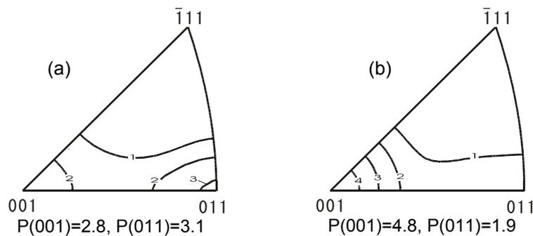
Fig. 4 Inverse pole figures showing the effect of strain on the components of the fiber texture constructed in Al-3Mg. The deformation was conducted at  $723\text{K}$  with a strain rate of  $5.0 \times 10^{-4} \text{s}^{-1}$ . The amounts of strain are (a)  $-1.0$  and (b)  $-1.4$ . Contour lines for the densities of compression axis are given. Mean density is used as a unit.  $P(001)$  and  $P(011)$  express the pole density at  $(001)$  and  $(011)$ , respectively.
