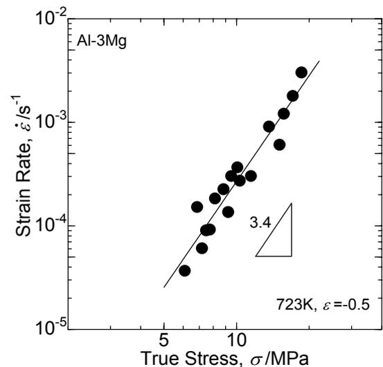
Fig. 2 True stress vs. strain rate relationship for Al-3Mg examined at a strain of -0.5. The deformation is conducted at 723K.
