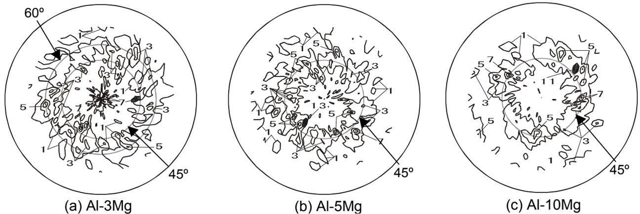
Fig. 3  $\{011\}$  pole figures for (a) Al-3Mg, (b) Al-5Mg, and (c) Al-10Mg alloys after the deformation up to a strain of  $-1.0$  at  $723\text{K}$  with a strain rate of  $5.0 \times 10^{-4} \text{s}^{-1}$ . Pole densities are projected onto the compression plane. Mean pole density is used as a unit for drawing the contours.
