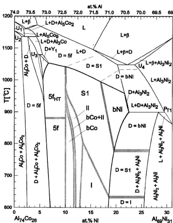
**Fig. 4** Experimentally determined partial Al-Ni-Co phase diagram along the composition line  $\text{Al}_{74}\text{Co}_{26} - \text{Al}_{69}\text{Ni}_{31}$  [13]. There are at least nine structural types of the decagonal quasicrystalline phases within this composition/temperature range. Note that even a few at.% difference in compositions causes a structural change.
