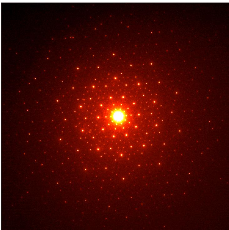
**Fig. 1** Precession electron diffraction pattern of the Al<sub>72</sub>Ni<sub>20</sub>Co<sub>8</sub> decagonal quasicrystal, one of the best quasiperiodic ordered materials available today.
