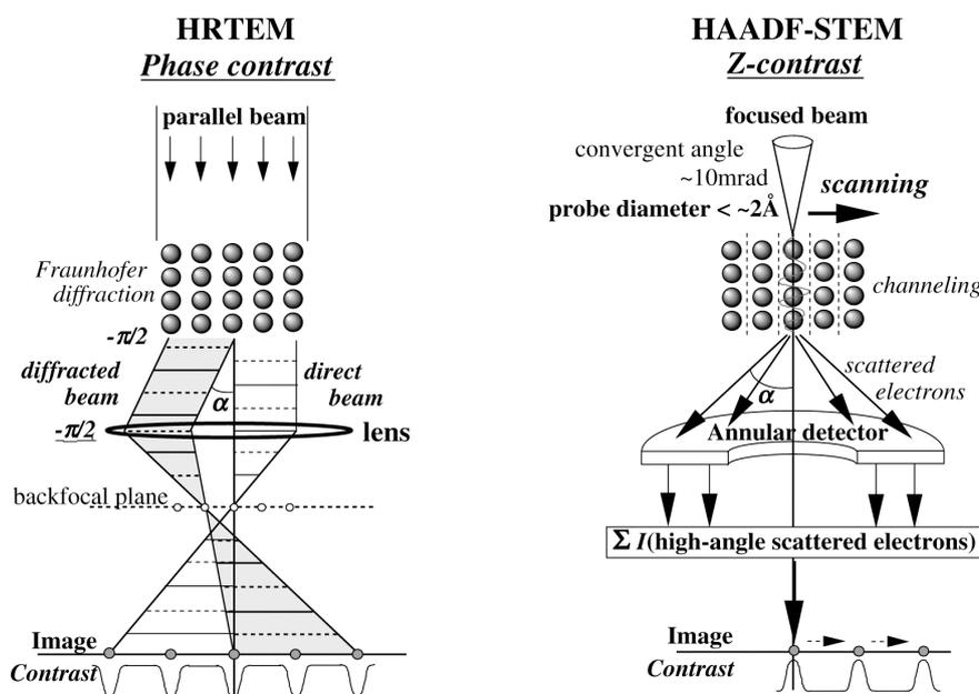
**Fig. 2** Schematic drawing of atomic-resolution imaging of high-resolution transmission electron microscopy (HRTEM, left) and scanning transmission electron microscopy (STEM, right). By capturing the scattered electron at high-angles with the annular detector, STEM provides significantly atomic-number dependence contrast (Z-contrast).
