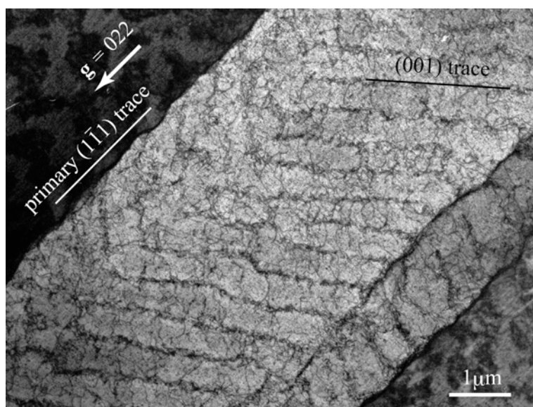
Fig. 2 Dislocation microstructure developed in a PSB of a specimen of aluminum single crystal cyclically deformed at \gamma_{pl} = 3 \times 10^{-3} until \gamma_{cum} = 96 at 77 K. The foil normal is close to [21\bar{1}] .
