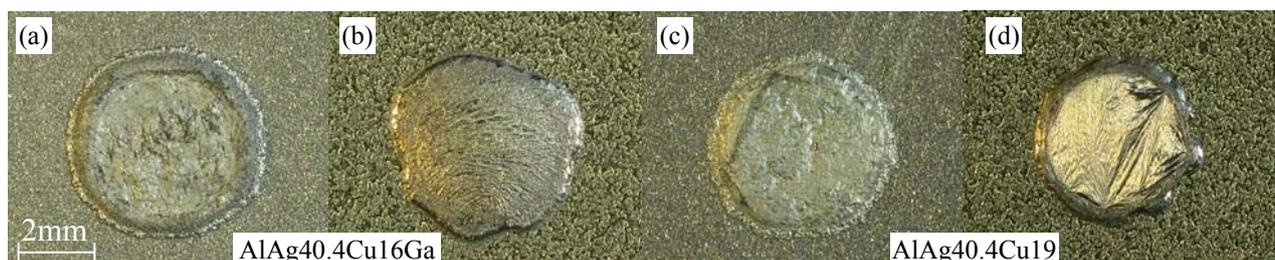
Figure 3: Wetting tests of Al-Ag-based filler metals on DC04
