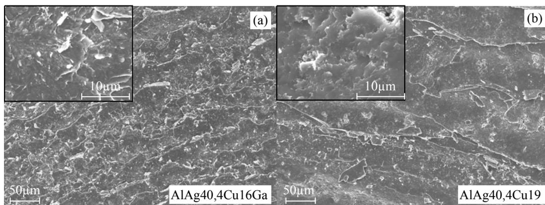
Figure 8: Fracture surfaces of the aluminum-steel-joints using Al-Ag-based filler metals
