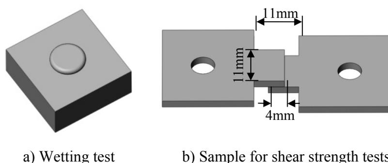
Figure 1: Applied spreading ability tests and strength test
