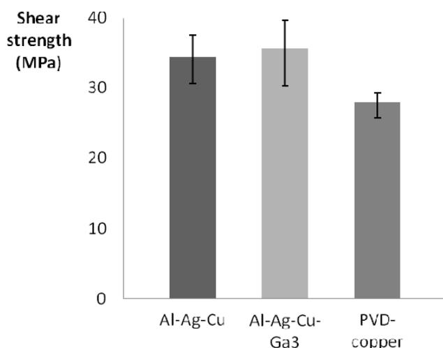
Figure 7: Shear strength of the brazements
