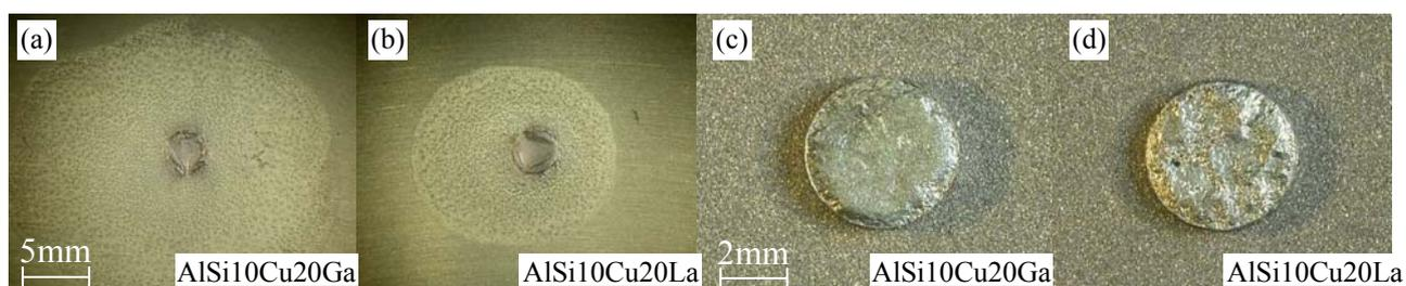
Figure 2: Wetting tests of Al-based filler metals on AW6060 (a, b) and on DC04 (c, d)
