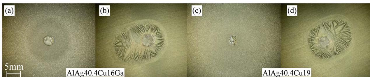
Figure 4: Wetting tests of Al-Ag-based filler metals on AW6060
