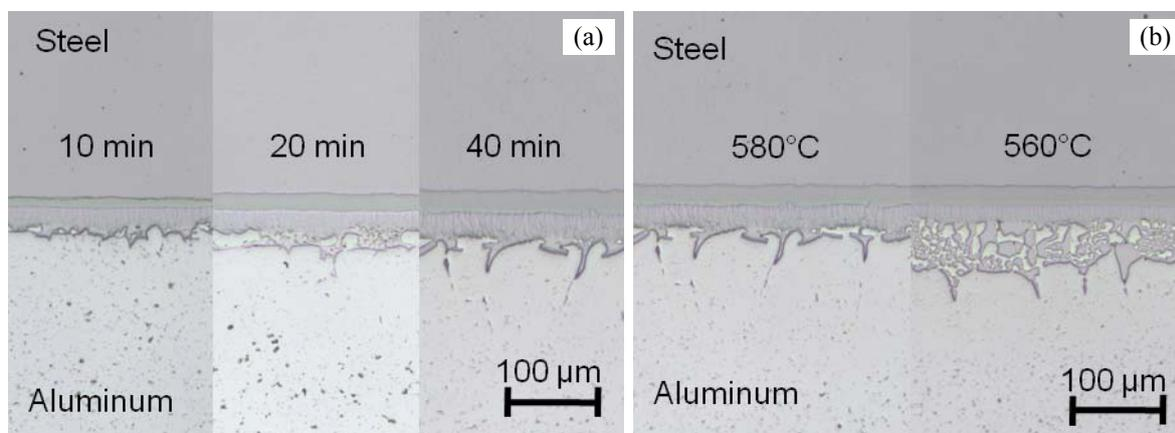
Figure 6: Micrographs of diffusion brazed aluminum/steel joints using arc-PVD coating varying dwell time at 580°C (a) and varying the brazing temperature at constant dwell time of 40 min (b)
