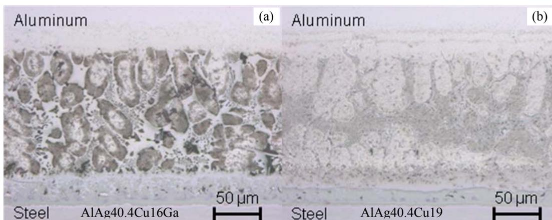
Figure 5: Micrograph of aluminum/steel joints brazed at 570°C using Al-Ag-based filler metals
