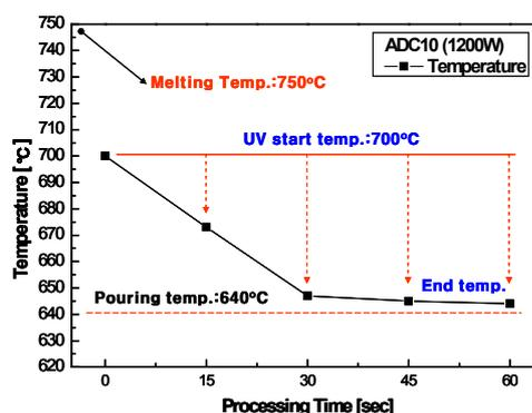
Fig. 6 Temperature variations of aluminum melts after ultrasonic treatment as a function of processing time.
