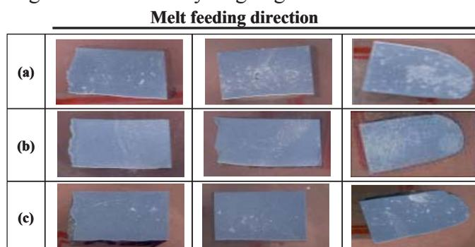
Fig. 2 Cross-section image of fluid test ALDC10 alloy as a function of processing time : (a) 0sec, (b) 15sec and (c) 30sec.
