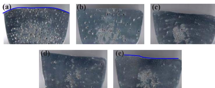
Fig.4 Cross-section image of RPT test ALDC10 alloy as a function of processing time : (a) 0sec, (b)15sec, (c) 30sec, (d)45sec and (e)60sec.
