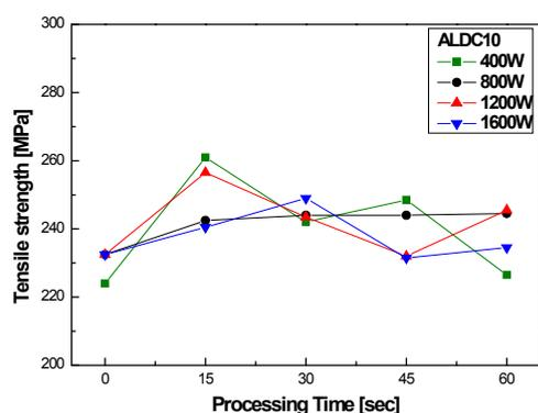
Fig. 5 Tensile strength of the ALDC10 alloy as a function of output power and processing time.
