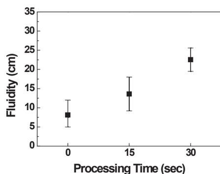
Fig. 1 Flow length of the ALDC10 alloy as a function of processing time.
