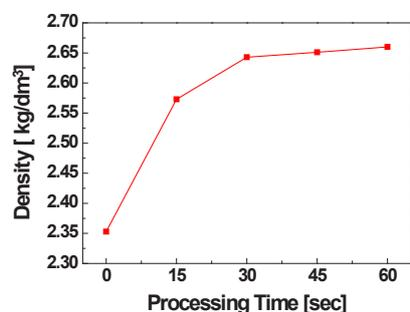
Fig.3 Density of the ALDC10 alloy as a function of processing time.
