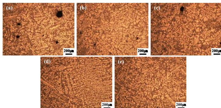
Fig. 7 Microstructure of tensile test ALDC10 alloy as a function of processing time : (a) 0sec, (b) 15sec, (c) 30sec, (d) 45sec and (e) 60sec
