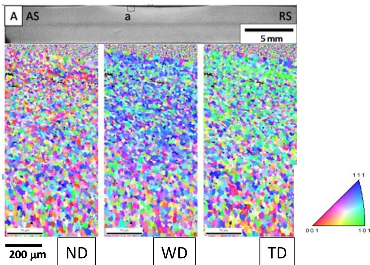
Fig. 3 Cross sectional view and inverse pole figure maps of friction stir welded 5083Al alloy joint. The EBSD data was taken from the black rectangular shown in the Fig.3(A).
