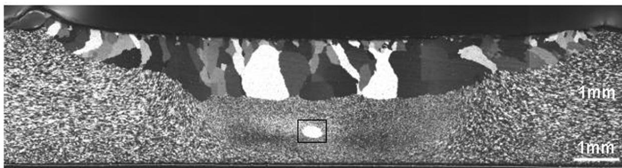
Fig.1 Abnormal grain growth observed at 823K in the joint of 5083 Al alloy friction stir processed at a rotation speed and a traveling speed of 800 rpm and 100mm/min., respectively.
