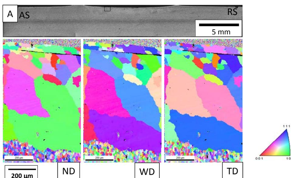
Fig.2 Cross sectional view and inverse pole figure maps of 5083Al alloy joint post-weld heat treated at 773K for 35s. The EBSD data was taken from the black rectangular shown in the Fig.2(A).
