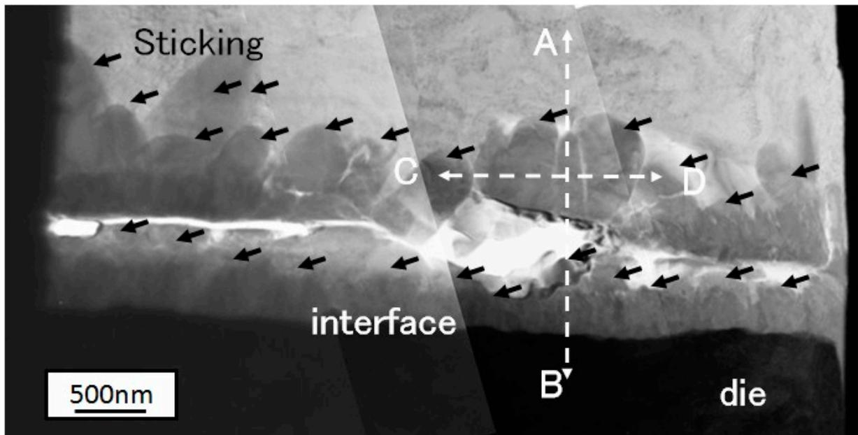
**Fig. 3:** TEM image of the interface between stacked #2 alloy and a die obtained for the sample prepared by FIB.
