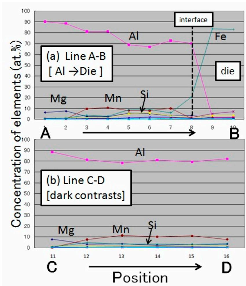
**Fig. 4:** Summary of EDS analysis obtained for TEM sample of #2 alloy in Fig. 3. (a) for line A-B through the interface and (b) for line C-D on the dark particles.
