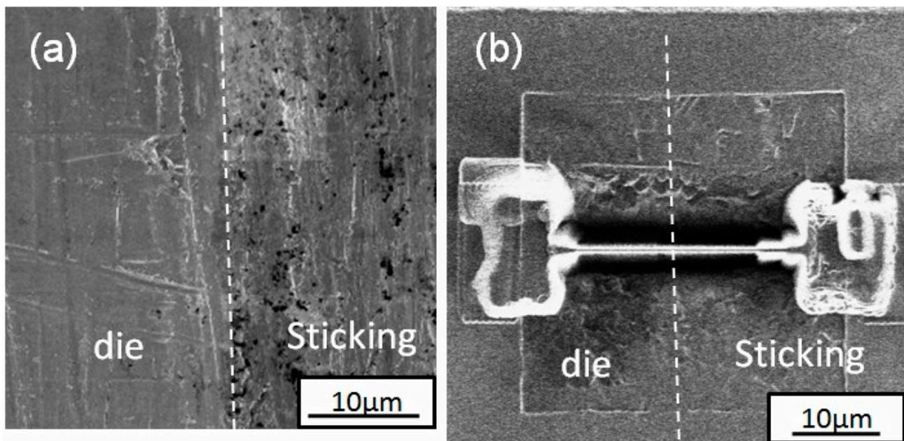
**Fig. 2:** (a) SEM image of the interface between stacked #2 alloy and a die and (b) secondary ion image by FIB at the same position as (a).
