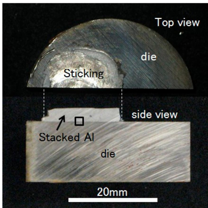
**Fig. 1:** Outlook of a cut die with sticking of #2 alloy.
