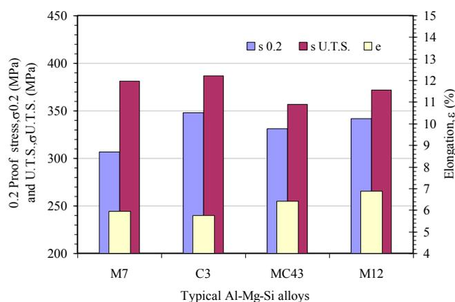
Fig. 5 Mechanical properties of Al-Mg-Si based alloys produced by the D-SSF process.
