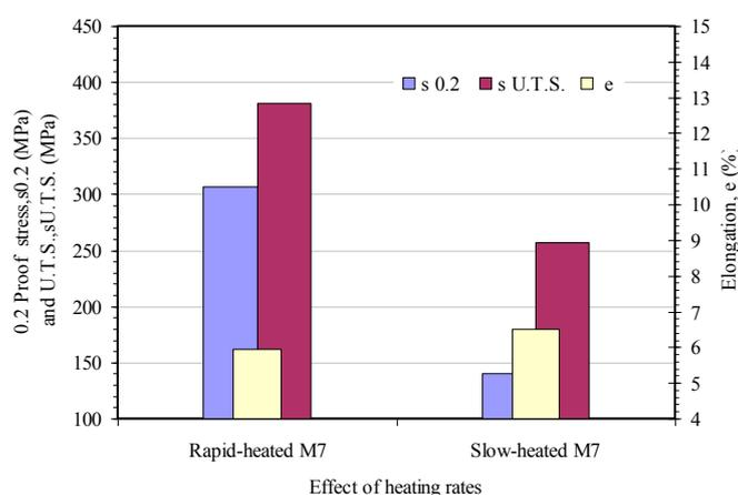
Fig. 4 Comparison of mechanical properties between the rapid-heated and slow-heated specimens of the D-SSF processed M7 alloy, showing higher strength in the rapid-heated specimen.
