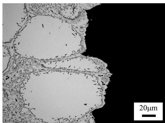
Fig. 6 Optical micrographs near fracture surfaces of M12 D-SSF processed alloys, showing the Mn dispersoid precipitate in  $\alpha$ -Al grains and solidified liquid phase regions.
