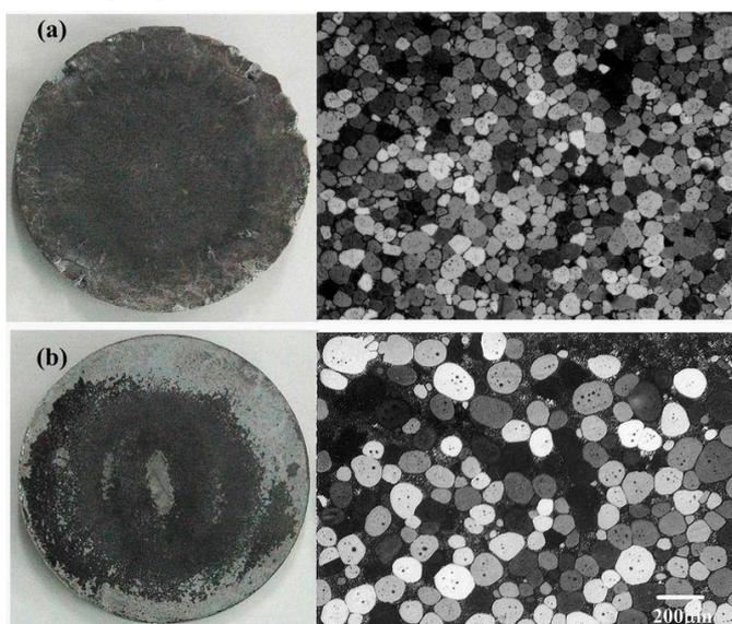
Fig. 3 Appearances and semi-solid microstructures of the D-SSF processed M12 alloy, showing (a) non-complete die-filling (low liquid fraction) of specimen heated of 637°C and (b) complete die-filling (high liquid fraction) of specimen heated of 646°C.
