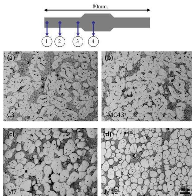
Fig. 2 Semi-solid microstructures of the D-SSF processed Al-Mg-Si based alloys from point No.2, (a) C3, (b) MC43, (c) M7 and (d) M12 alloys.
