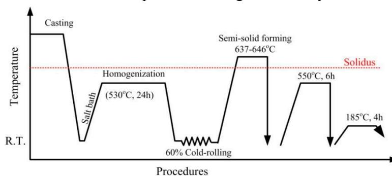
Fig. 1 Schematic illustration of the D-SSF process for Al-Mg-Si based alloys, showing casting, homogenization, semi-solid forming, solution treatment and aging processes.
