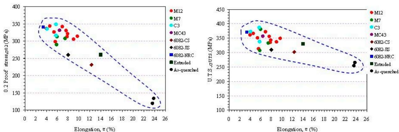
Fig. 11 0.2% proof stress and U.T.S. of the D-SSF processed alloys are shown inside a dotted line.
