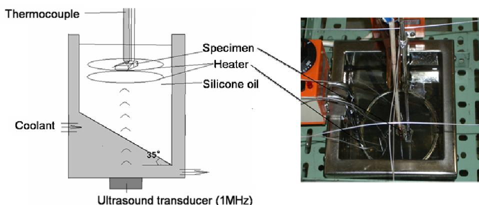
Fig.1 Schematic illustration and outlook of the ultrasound bath utilized in this work.
