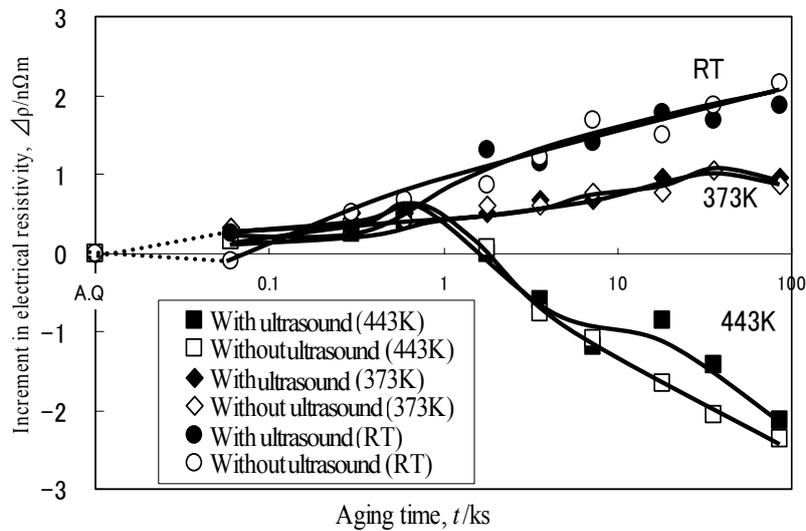
Fig.3 Increment in electrical resistivity of the specimens with and without ultrasound treatment at RT, 373 and 443K.
