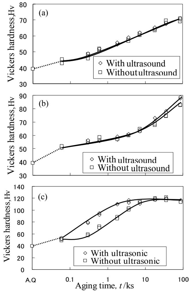
Fig.2 Age-hardening curves of the specimens with and without ultrasound treatment at (a)RT, (b)373K and (c)443K.
